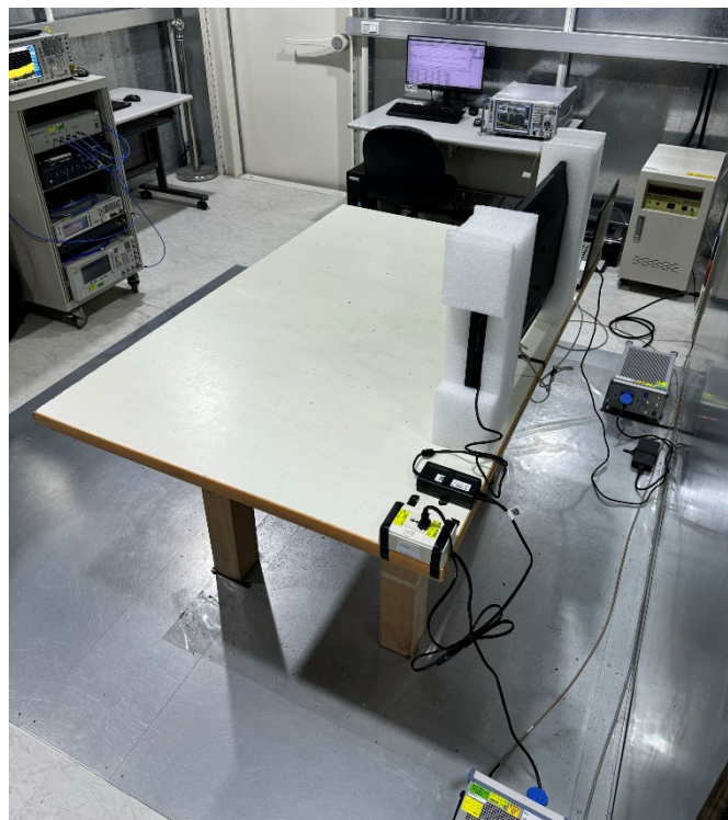
Back View of AC Power Line Conducted Emission Test
