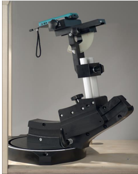
F-2. Device Holder for Transmitters
