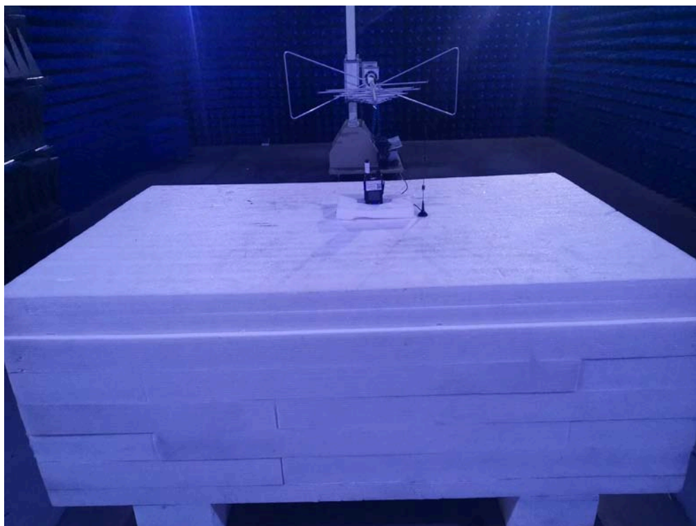
Photo of Radiated Emission Measurement (Above 1G)
