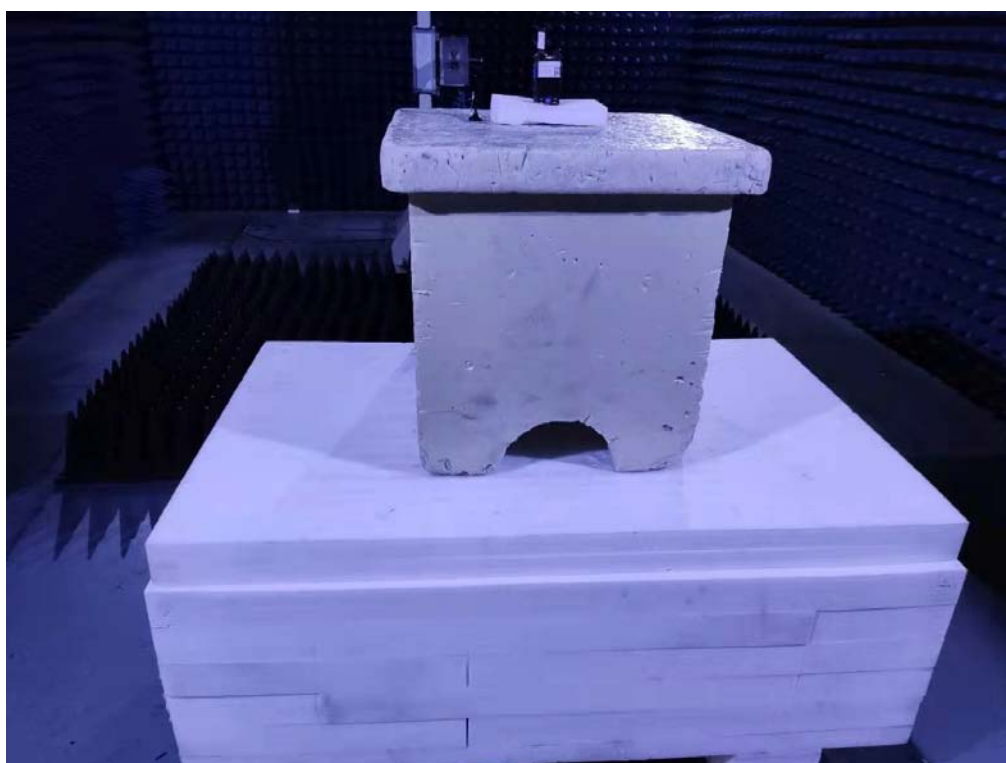
Photo of Radiated Emission Measurement (Above 1G)
