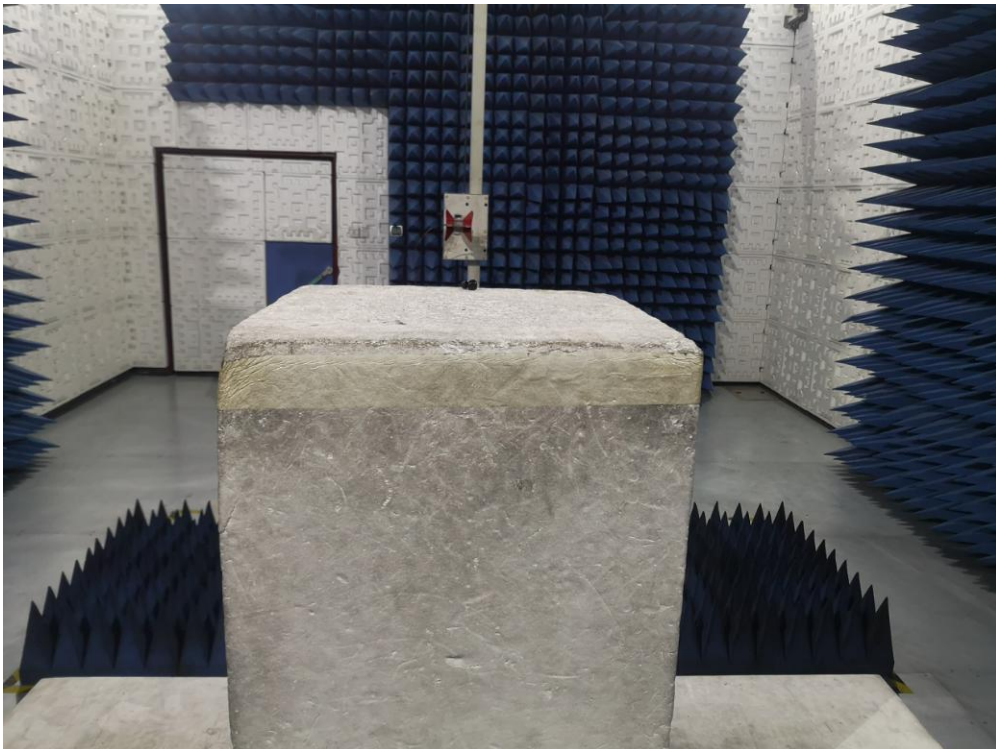
RADIATED EMISSION TEST SETUP ABOVE 1GHz
