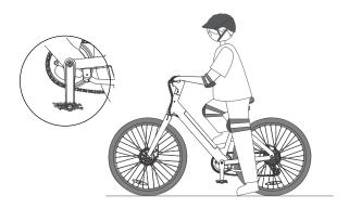
6. To reduce speed, gradually stop pedaling and squeeze the brake lever gently to brake. (Left brake lever controls front wheel braking, right brake lever controls rear wheel braking.)
