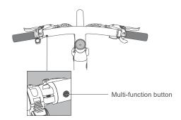
Gear shift: Short press the Multi-function button twice to shift 0-3 gear;
