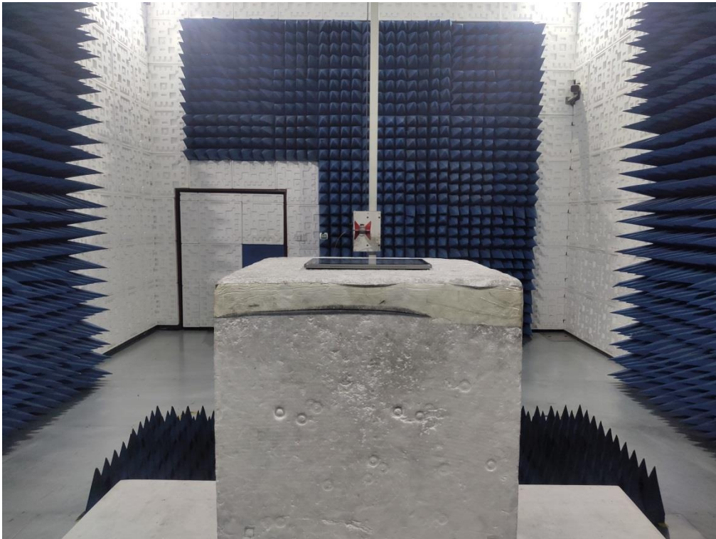
RADIATED EMISSION TEST SETUP ABOVE 1GHZ
