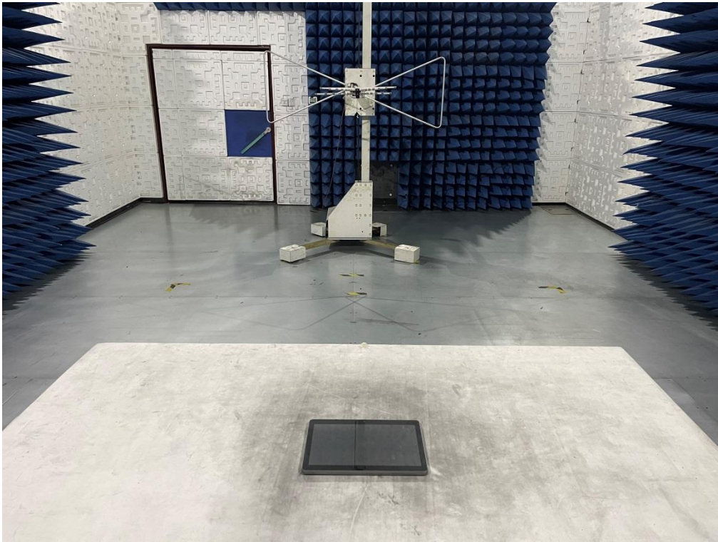
RADIATED EMISSION TEST SETUP ABOVE 1GHZ
