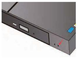
Press button in this hole with a needle and hold more than 2 seconds then release, CDRip will be reset.
