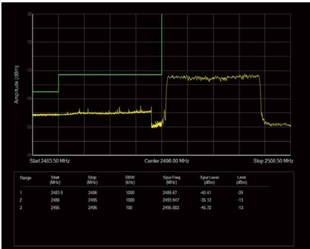
Band41 QAM16 BW=10MHz Channel=39700 RB Size=1 Position=#0
