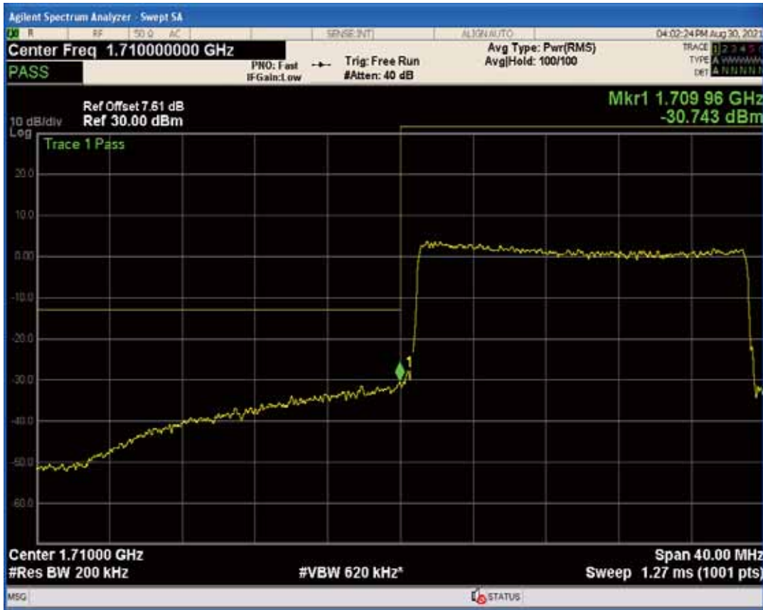
Band66 QPSK BW=20MHz Channel=132572 RB Size=1 Position=#0
