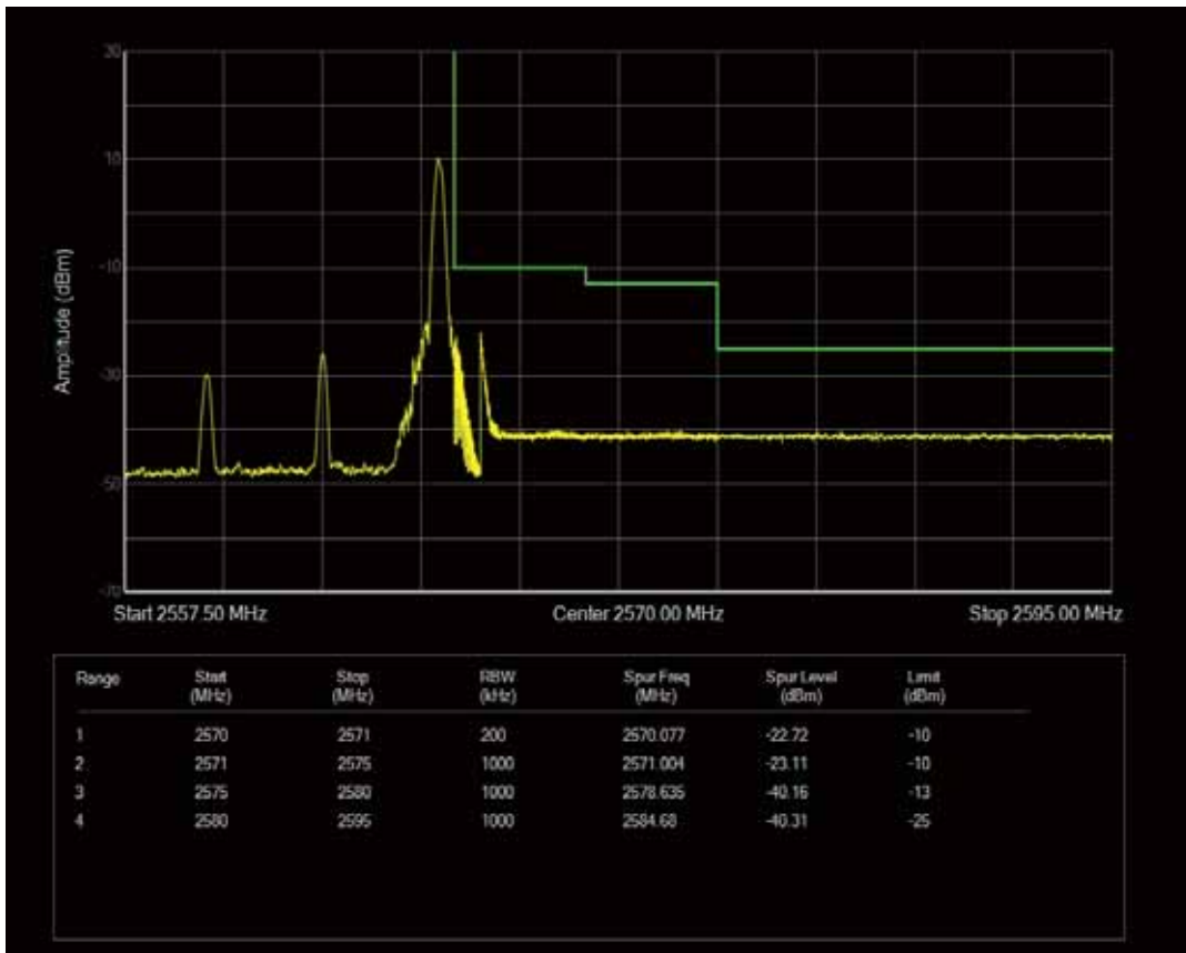
Band7 QPSK BW=10MHz Channel=21400 RB Size=1 Position=#0
