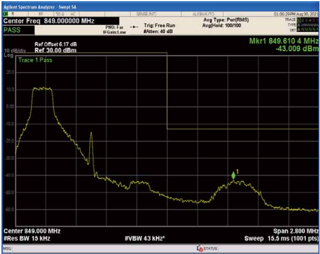
Band5 QAM16 BW=1.4MHz Channel=20643 RB Size=1 Position=#Max
