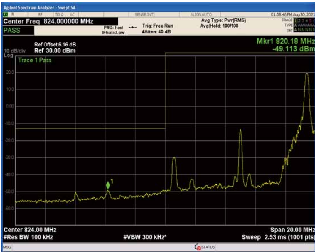
Band5 QAM16 BW=10MHz Channel=20450 RB Size=1 Position=#0
