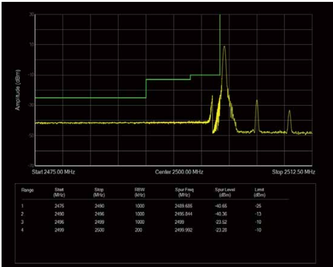
Band7 QPSK BW=10MHz Channel=20800 RB Size=50 Position=#0
