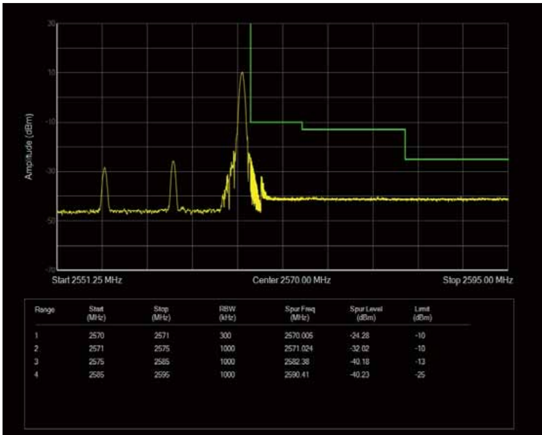
Band7 QAM16 BW=15MHz Channel=21375 RB Size=1 Position=#0
