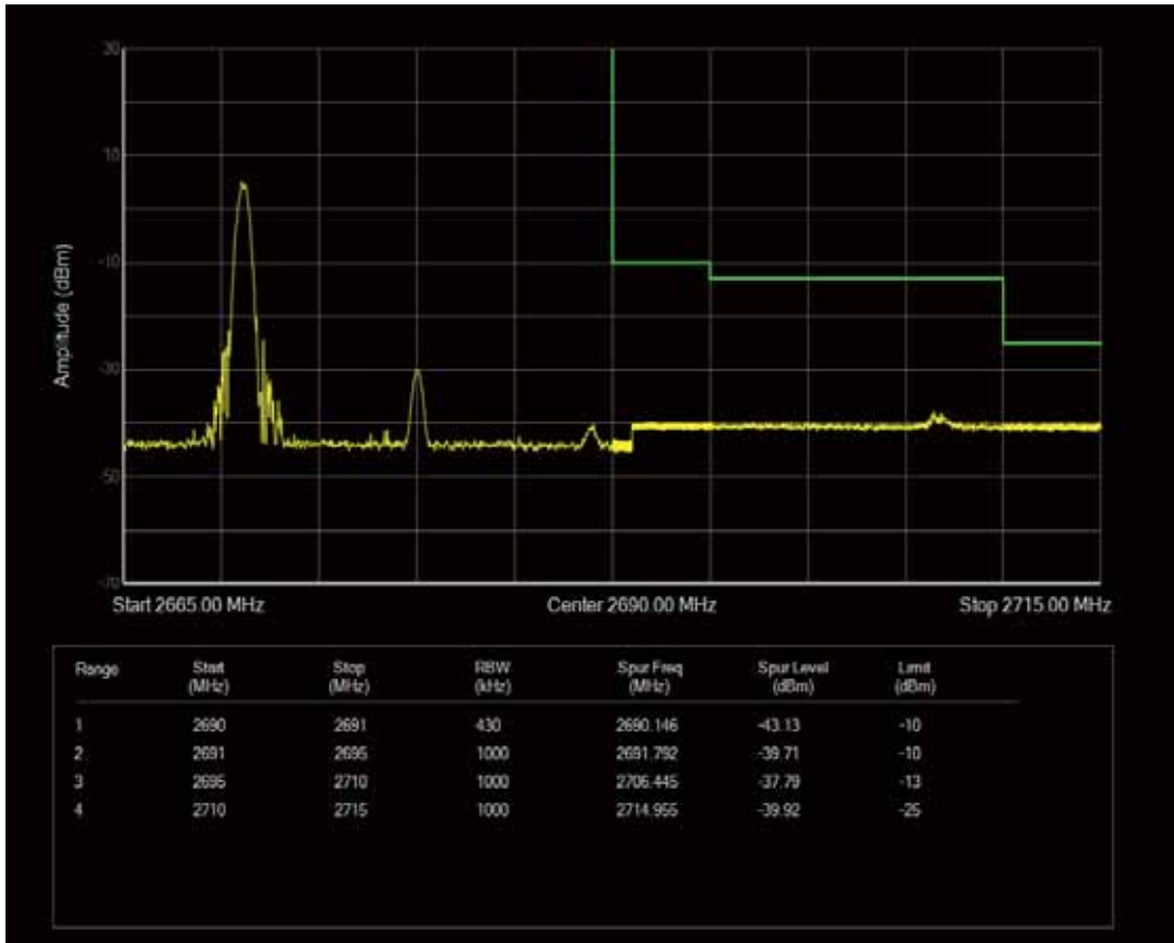
Band41 QAM16 BW=20MHz Channel=41490 RB Size=100 Position=#0
