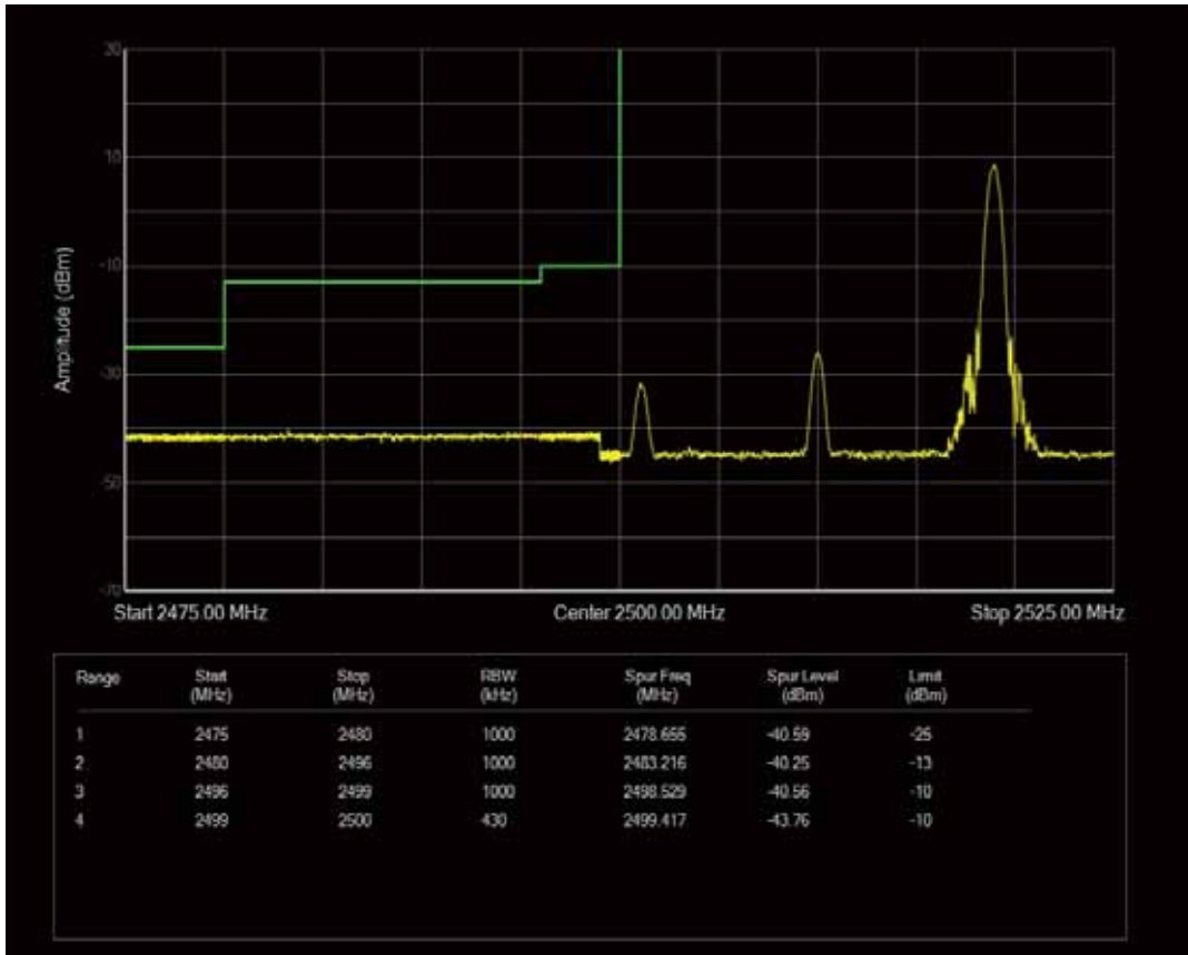
Band7 QAM16 BW=20MHz Channel=20850 RB Size=1 Position=#0
