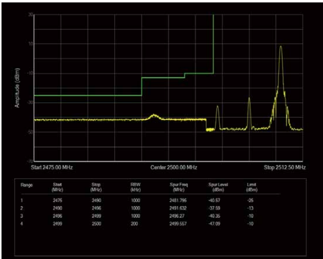
Band7 QAM16 BW=10MHz Channel=20800 RB Size=1 Position=#0
