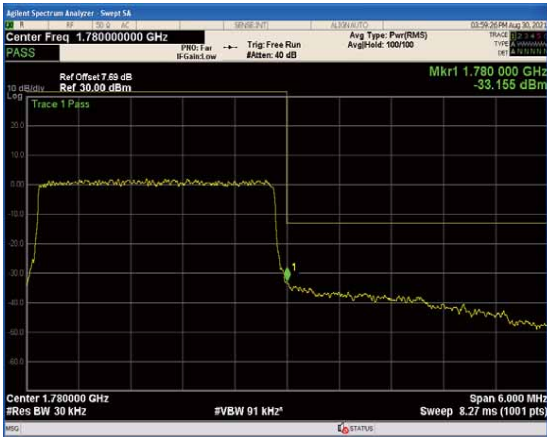
Band66 QAM16 BW=3MHz Channel=132657 RB Size=1 Position=#Max
