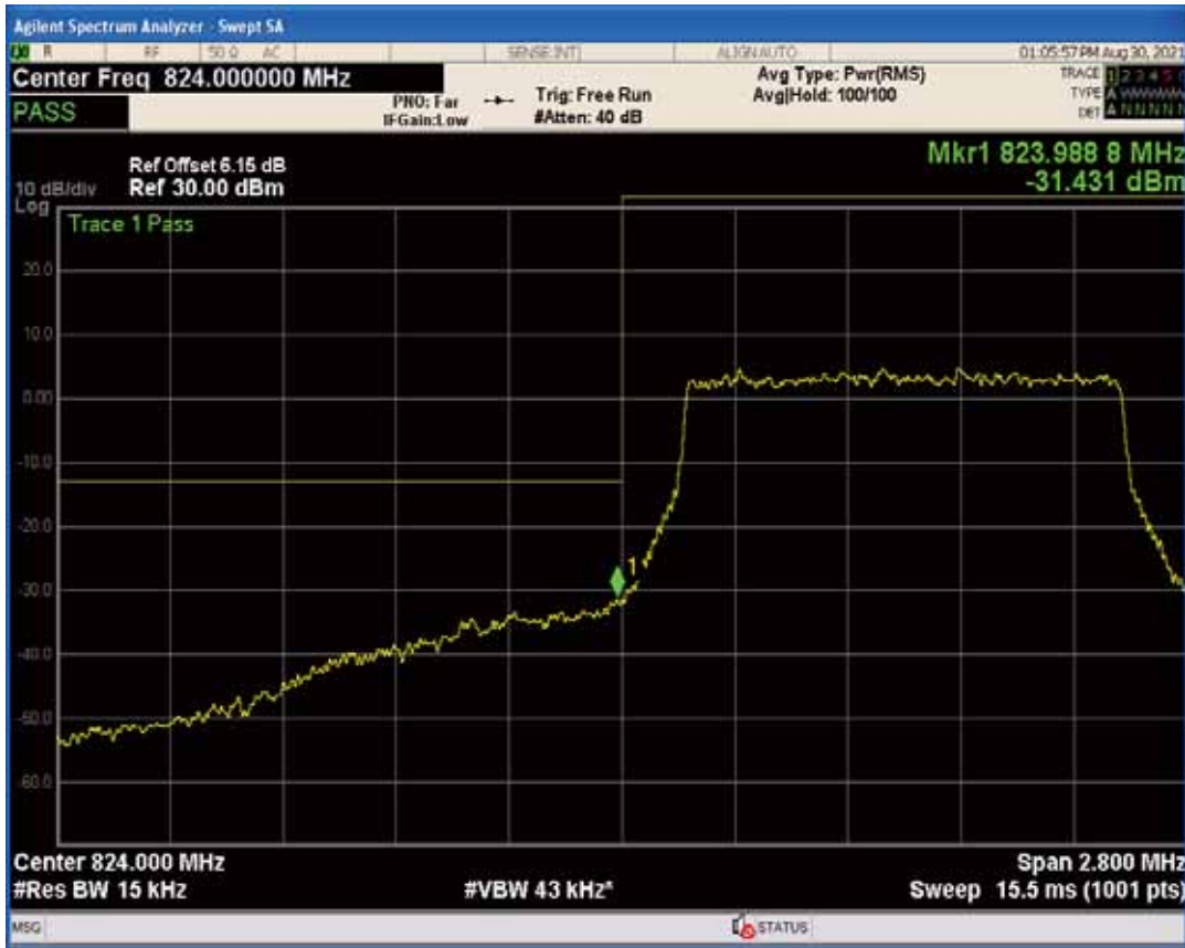
Band5 QPSK BW=1.4MHz Channel=20407 RB Size=1 Position=#Max
