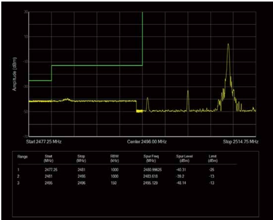
Band41 QPSK BW=15MHz Channel=39725 RB Size=1 Position=#0
