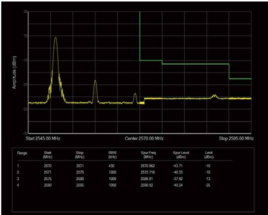
Band7 QPSK BW=20MHz Channel=21350 RB Size=100 Position=#0
