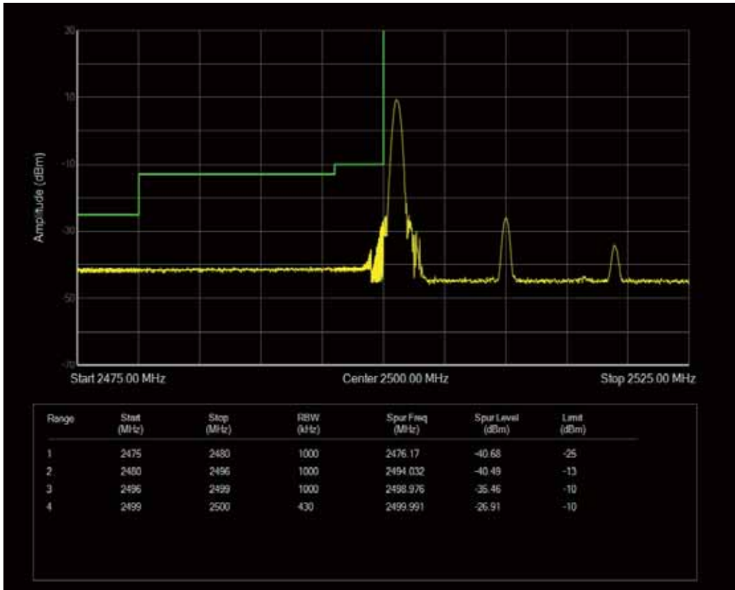
Band7 QPSK BW=20MHz Channel=20850 RB Size=100 Position=#0
