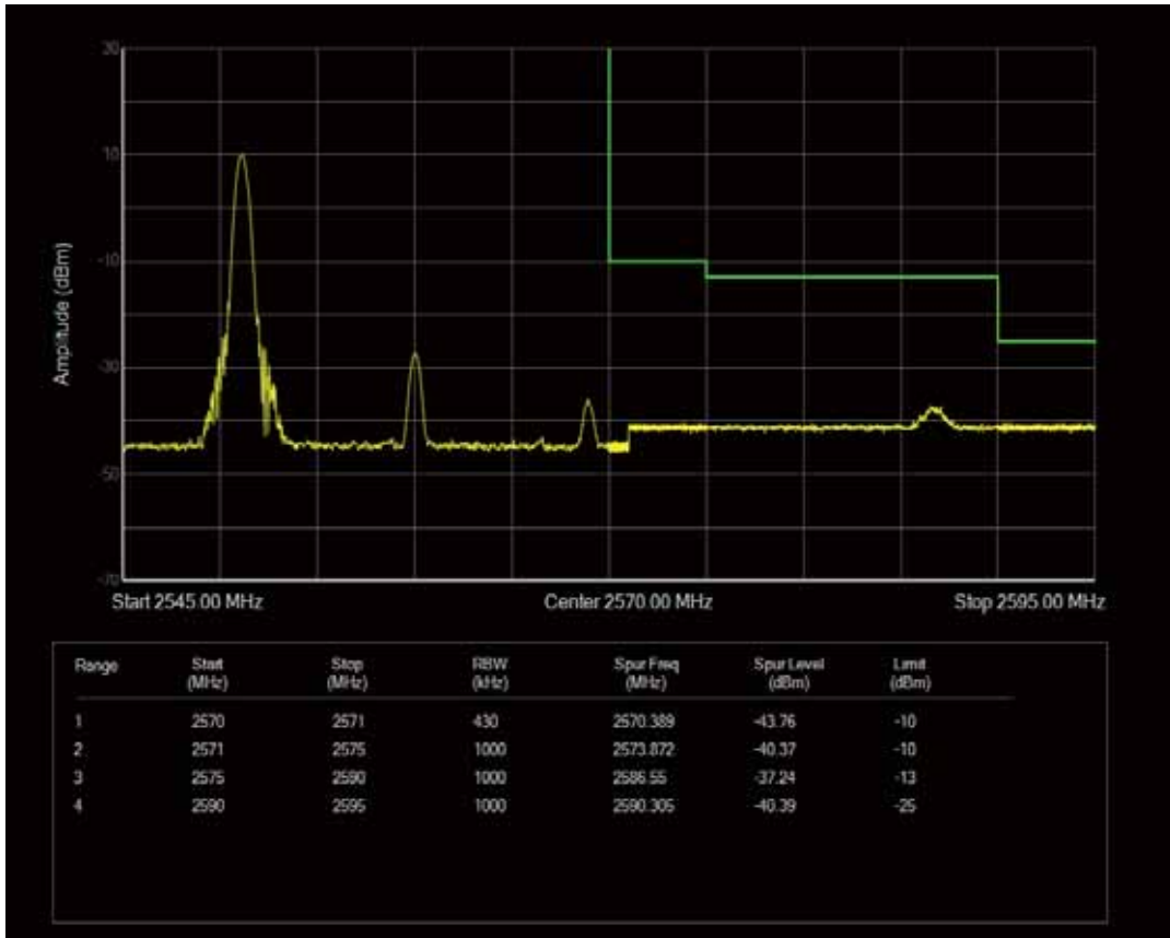
Band7 QAM16 BW=20MHz Channel=20850 RB Size=100 Position=#0
