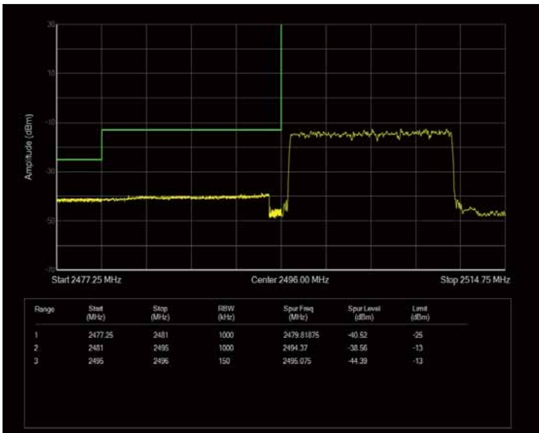
Band41 QAM16 BW=15MHz Channel=39725 RB Size=1 Position=#0
