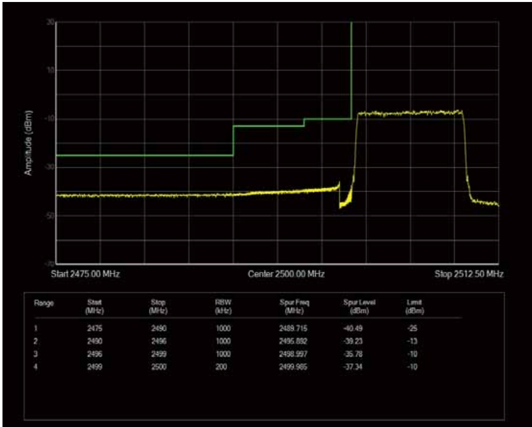
Band7 QPSK BW=10MHz Channel=20800 RB Size=1 Position=#Max
