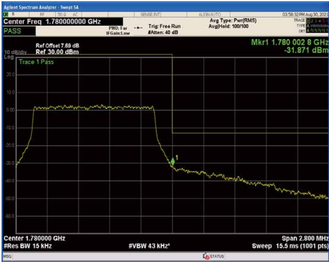
Band66 QPSK BW=3MHz Channel=131987 RB Size=1 Position=#Max
