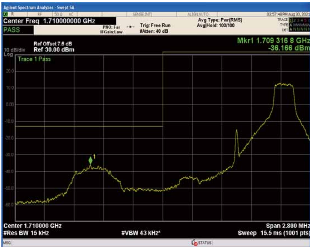
Band66 QPSK BW=1.4MHz Channel=131979 RB Size=1 Position=#0
