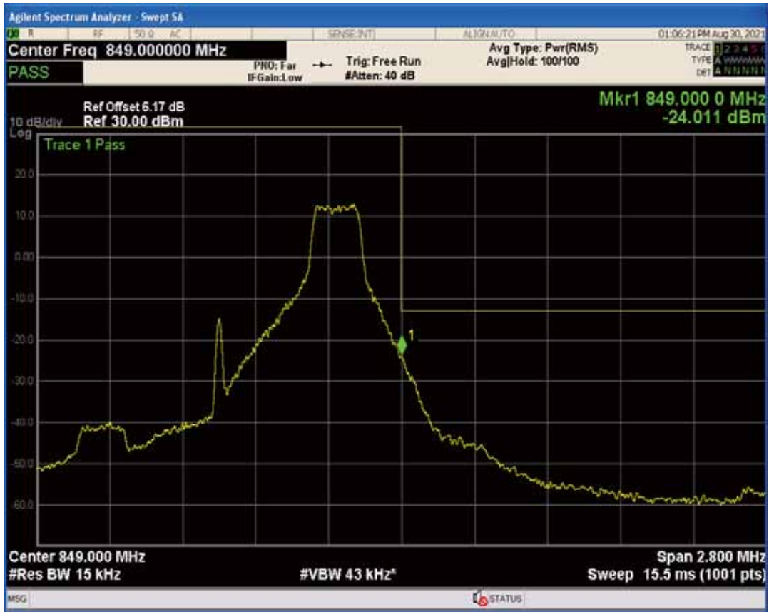
Band5 QPSK BW=1.4MHz Channel=20643 RB Size=6 Position=#0
