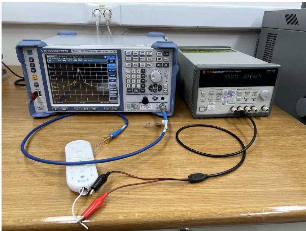
**- Radiated Emission Test (Below 1 GHz)**
