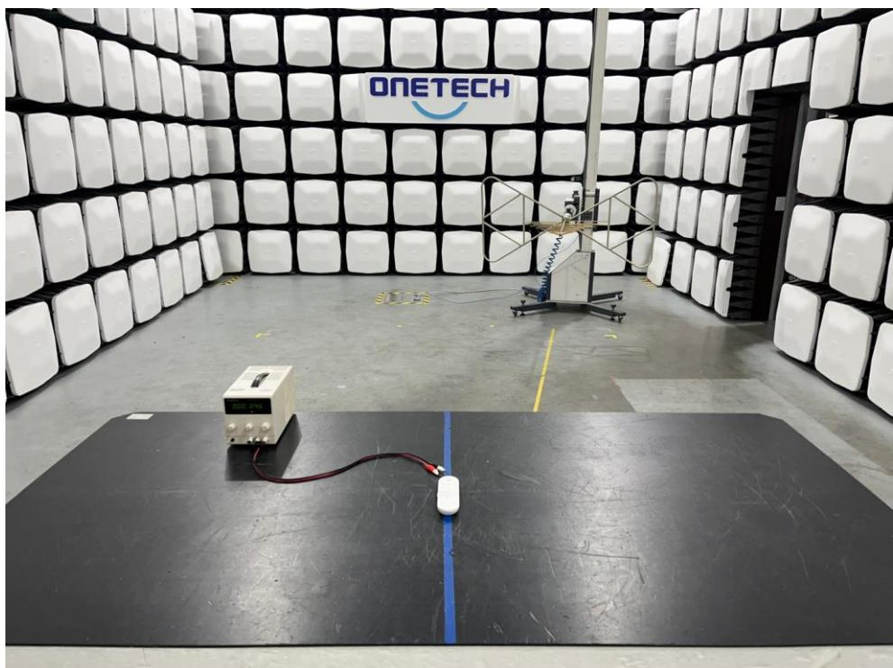
**- Radiated Emission Test (Above 1 GHz)**
