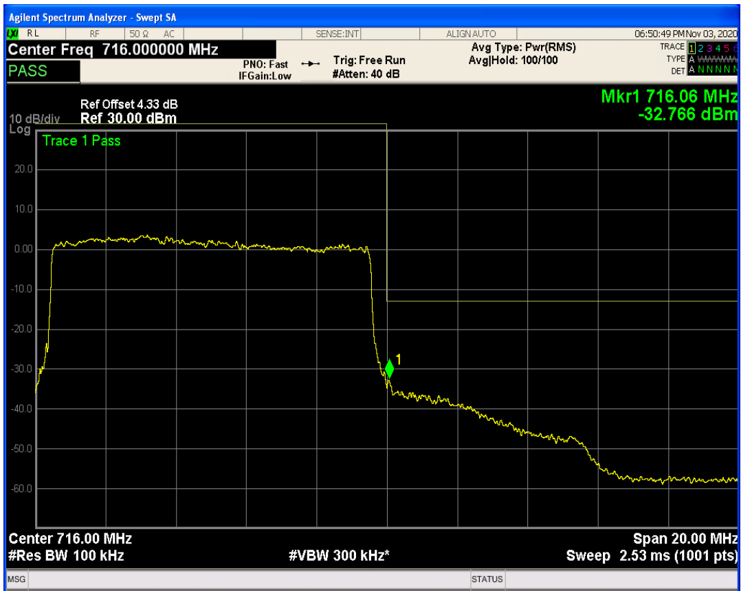
LTE Band17 QAM16 BW=10MHz Channel=23800 RB Size=1 Position=#0
