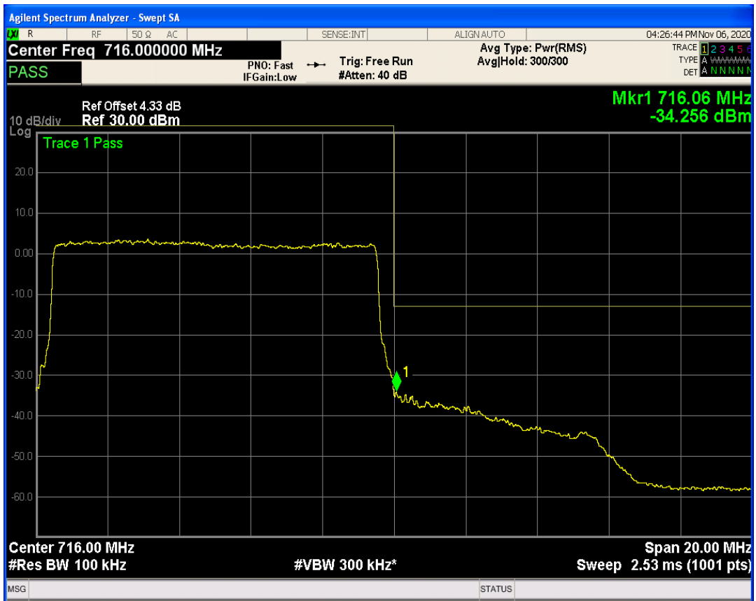
LTE Band12 QAM16 BW=10MHz Channel=23130 RB Size=1 Position=#0
