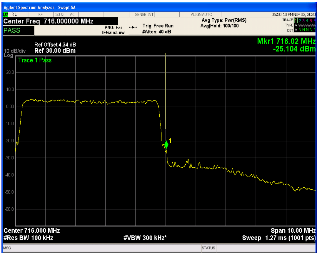
LTE Band17 QPSK BW=10MHz Channel=23780 RB Size=1 Position=#Max
