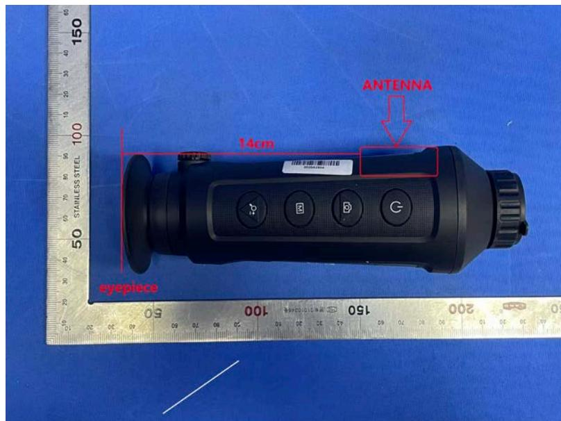
Note 1) The distance between WIFI antenna and eyepiece of the EUT is 140mm.
