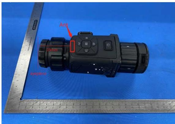
Note 1) The distance between WIFI antenna and eyepiece of the EUT is 25mm.
