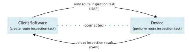
Figure 5-1 Route Inspection Work Flow
