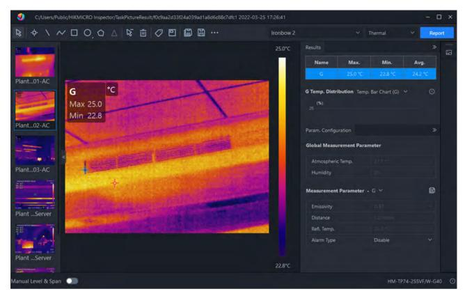
Figure 5-5 Analysis in HIKMICRO Analyzer
