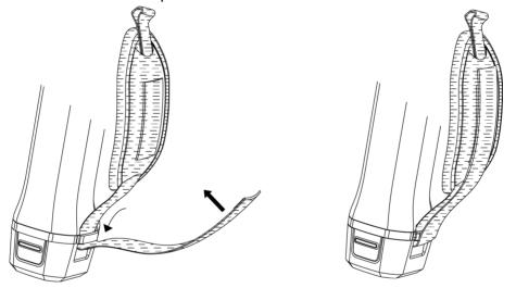
**Figure 2-4 Secure Lower Part of Hand Strap**
