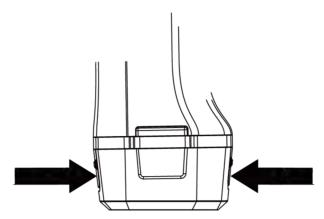
Figure 2-1 Remove Battery Base
