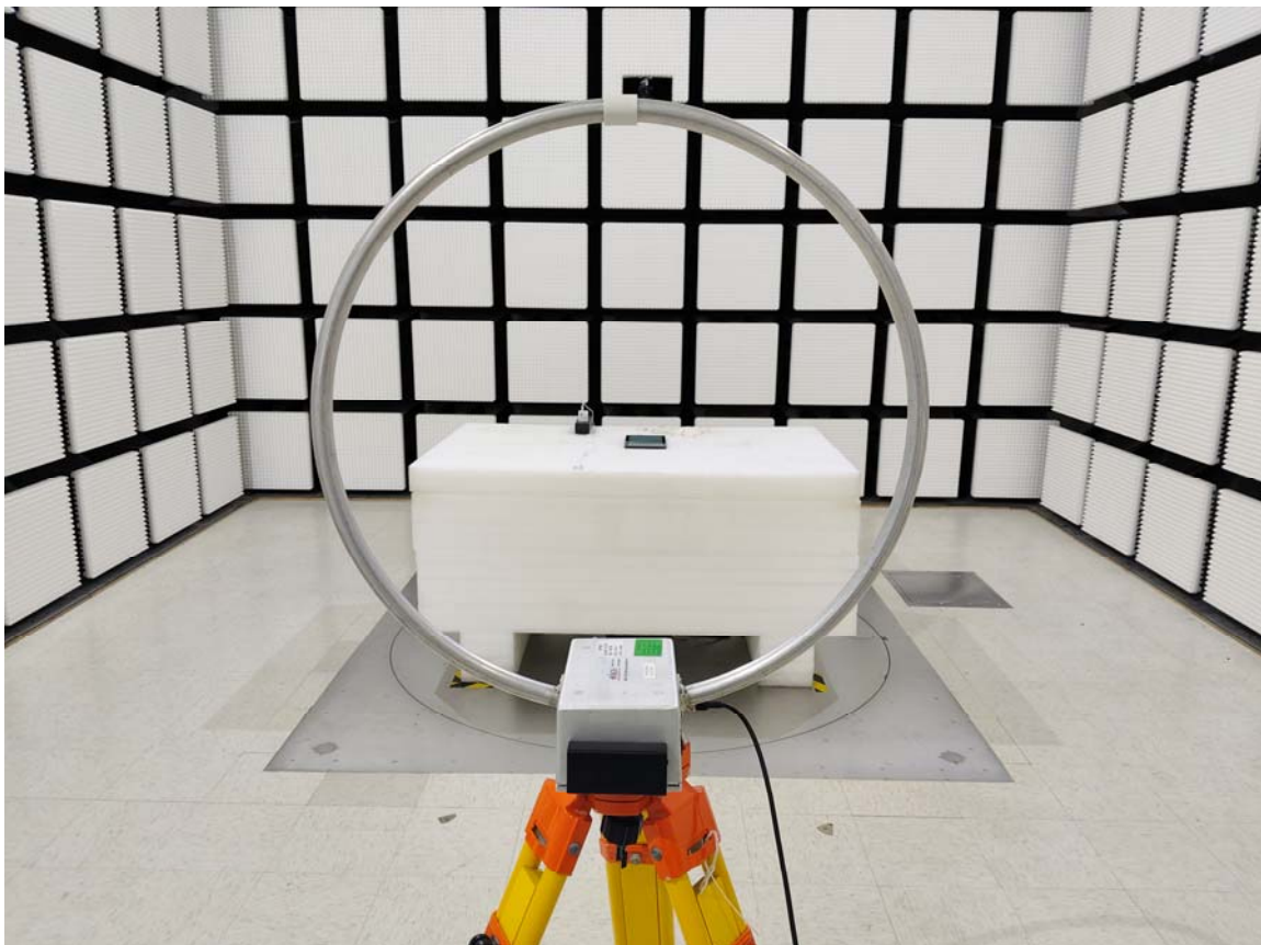
Radiated Emission 9 kHz-30 MHz Parallel View
