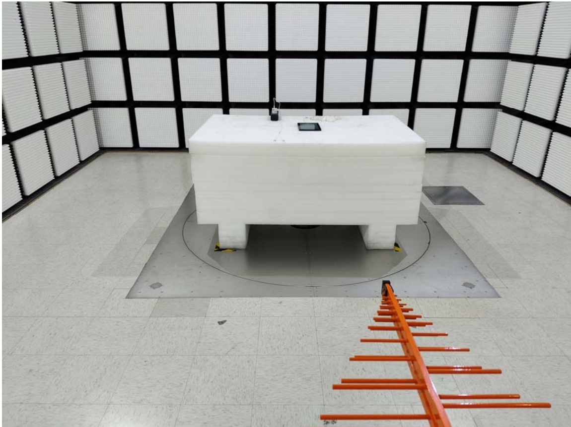
Radiated Emission 9 kHz-30 MHz Parallel View
