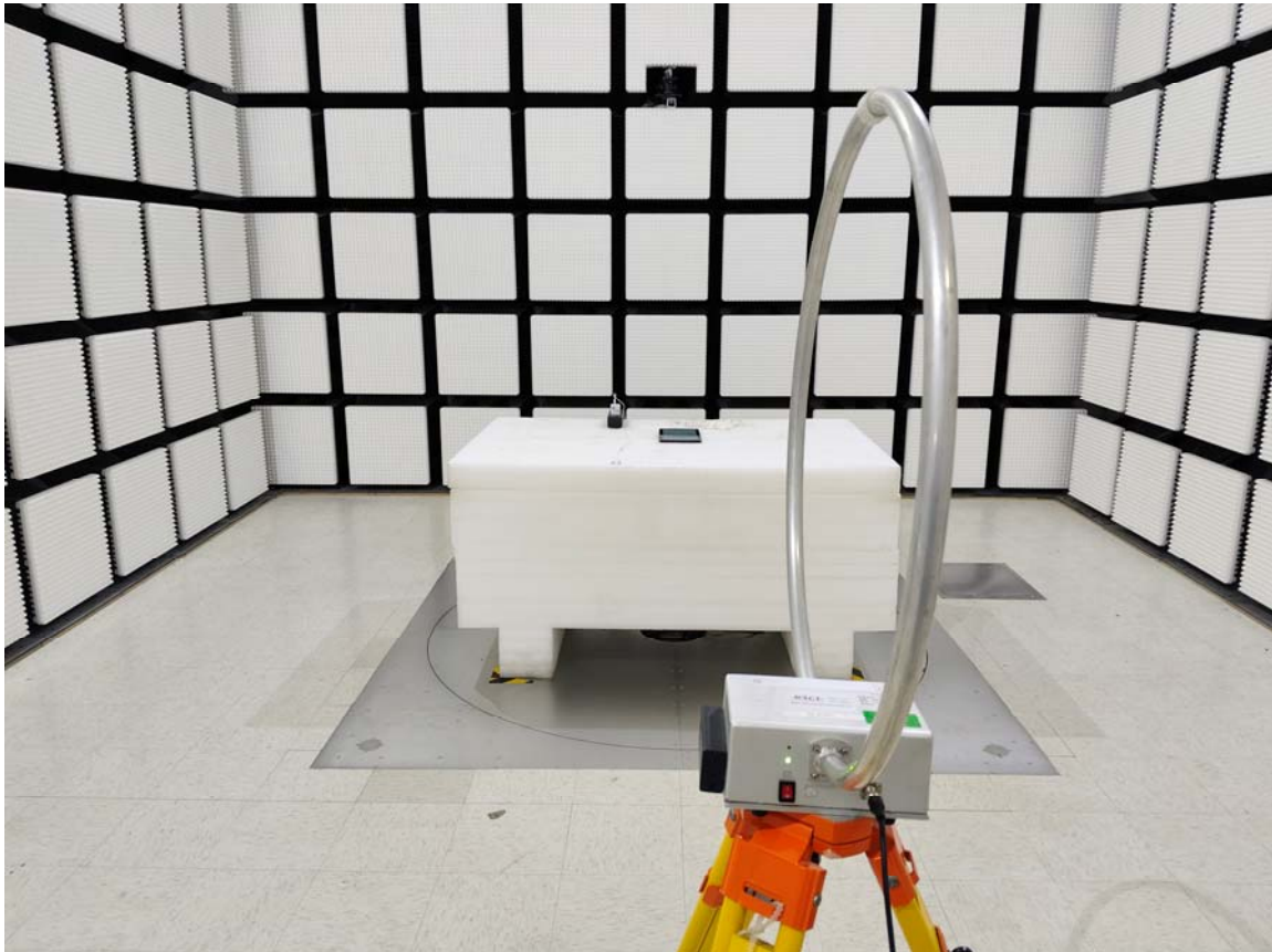
Radiated Emission 9 kHz-30 MHz Ground-parallel View
