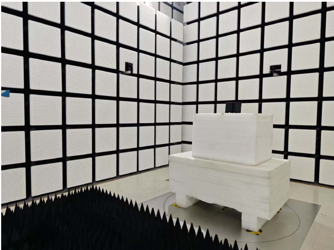
Radiated Emission 18-25 GHz View
