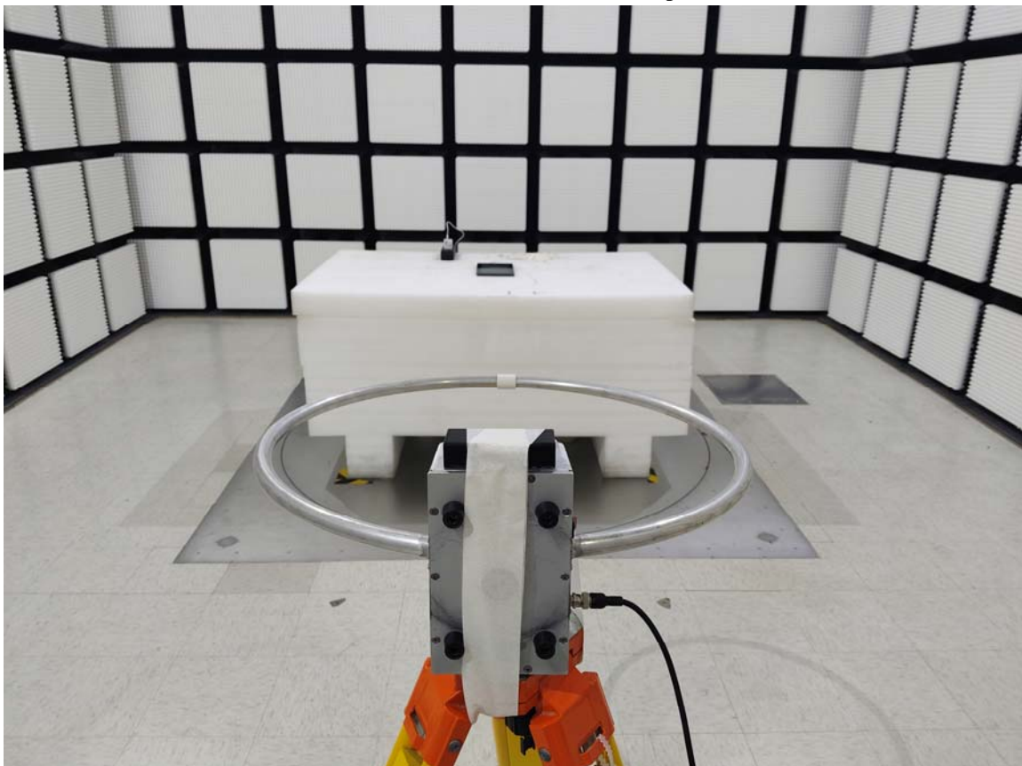
Radiated Emission 9 kHz-30 MHz Ground-parallel View
