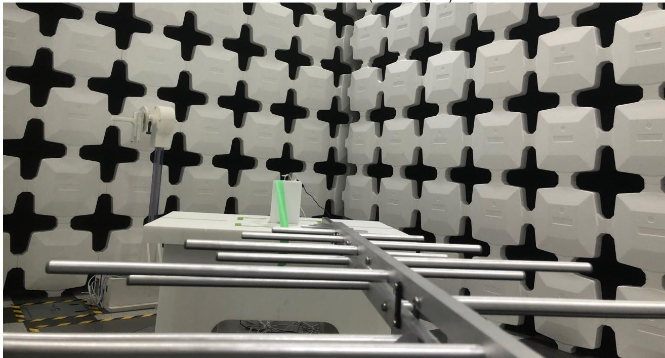
3. Radiated Measurement (Above 1GHz) Photo
