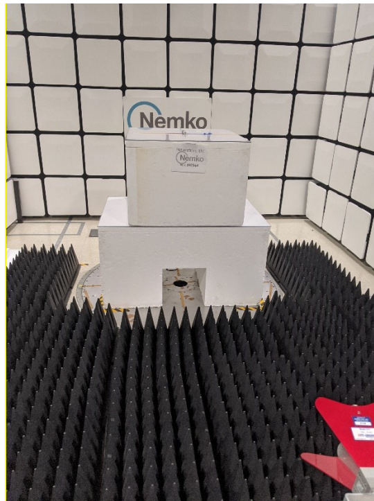
Figure 3 - Radiated emissions above 1 GHz, front view
