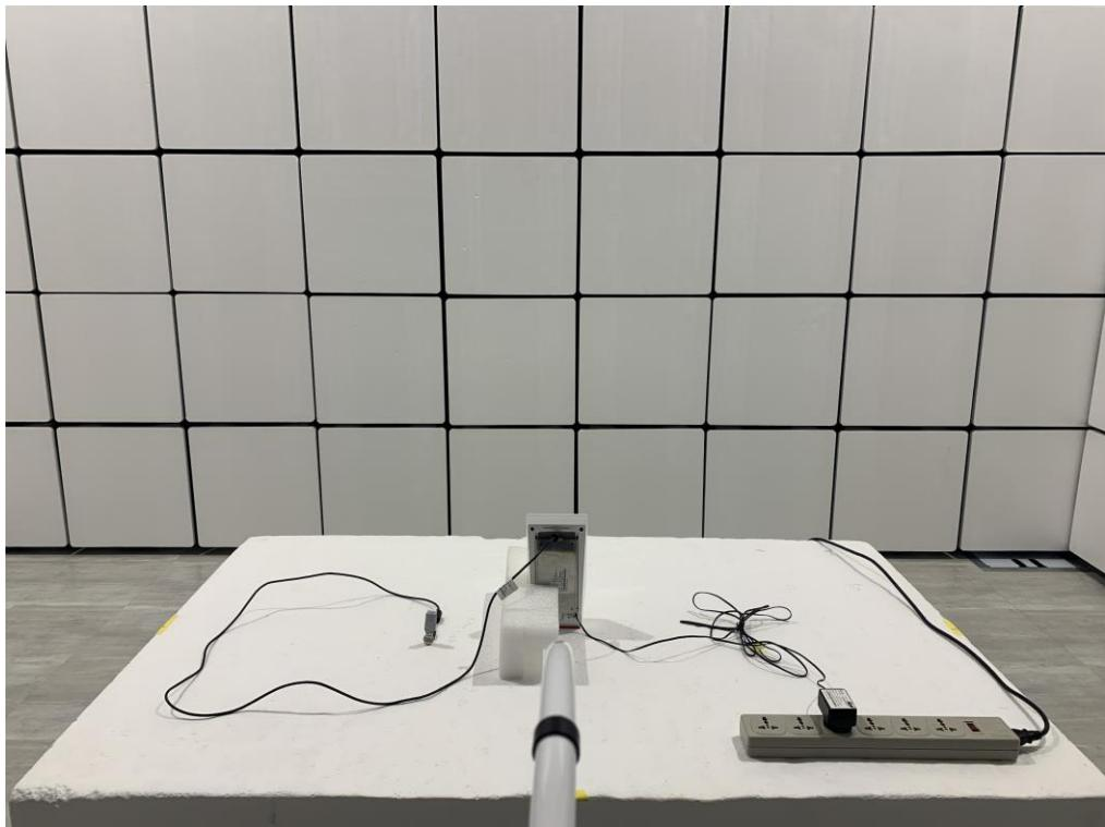
**Radiated emissions test photos****30 MHz to 1 GHz**
