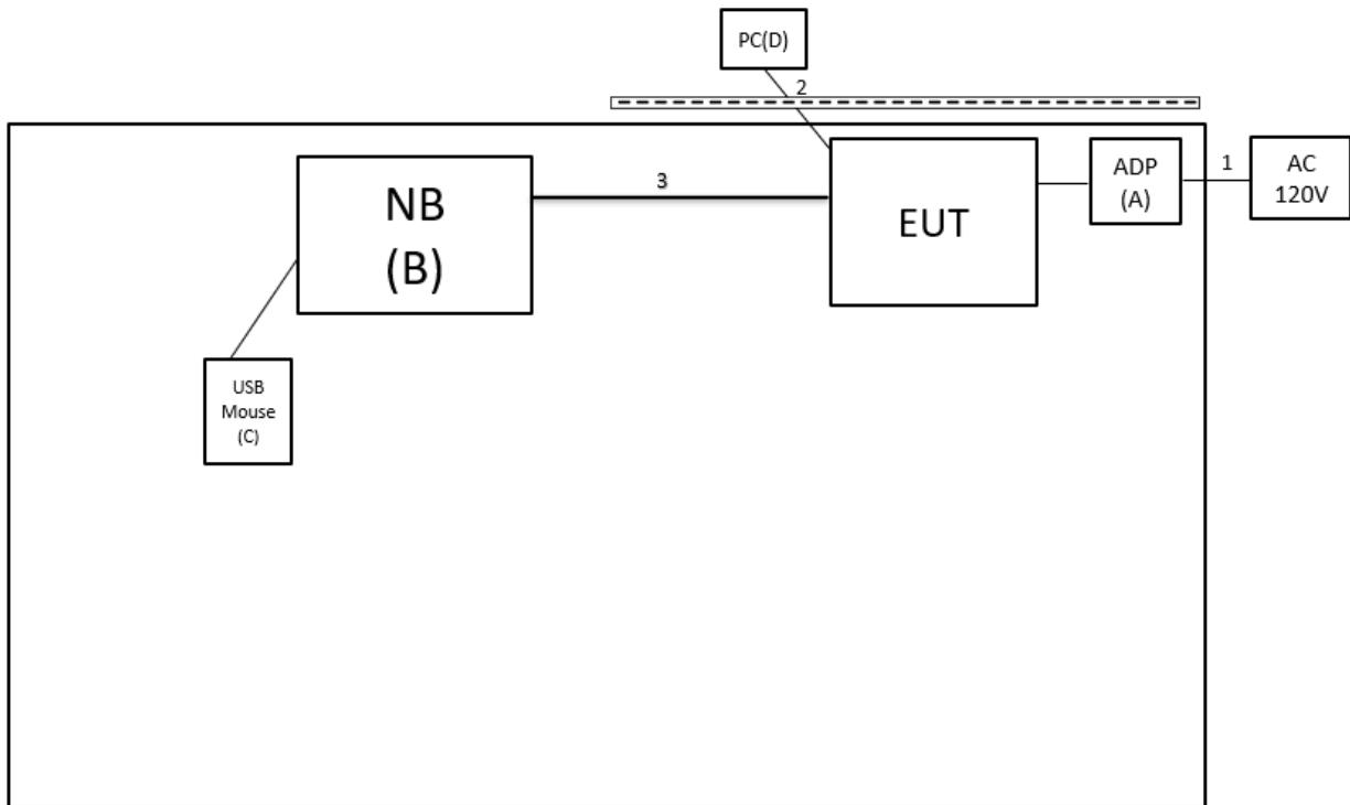
Radiated Emissions Test
