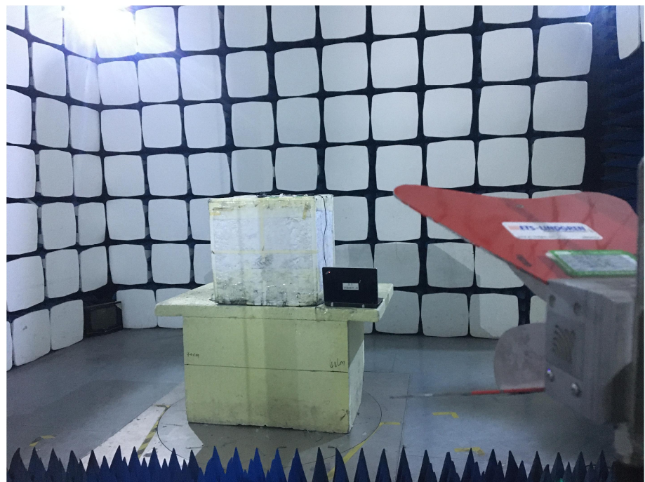
Radiation Emission Test Setup (1GHz to 18GHz)
