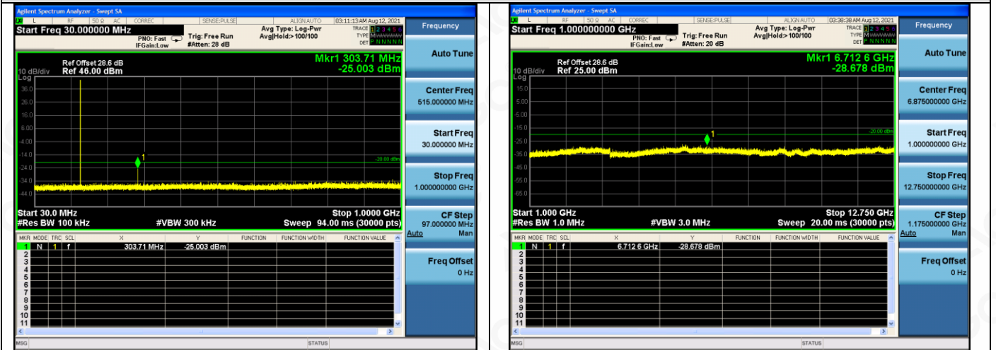
12.5kHz, Analog modulation, Assigned Frequency:155.7525MHz, 25W
