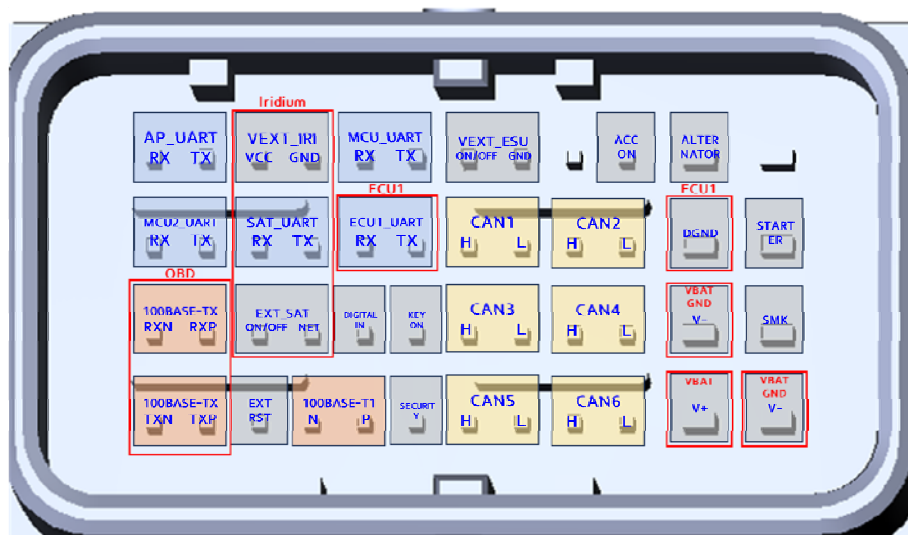
Fig. 3.7 Main Connector PINMAP1
