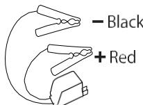
Jumper cables have designated colors, RED for POSITIVE (+) and BLACK for NEGATIVE (-). DO NOT allow the metal ends to touch together, this may harm the battery, charging system and/or electronics in the vehicle.
