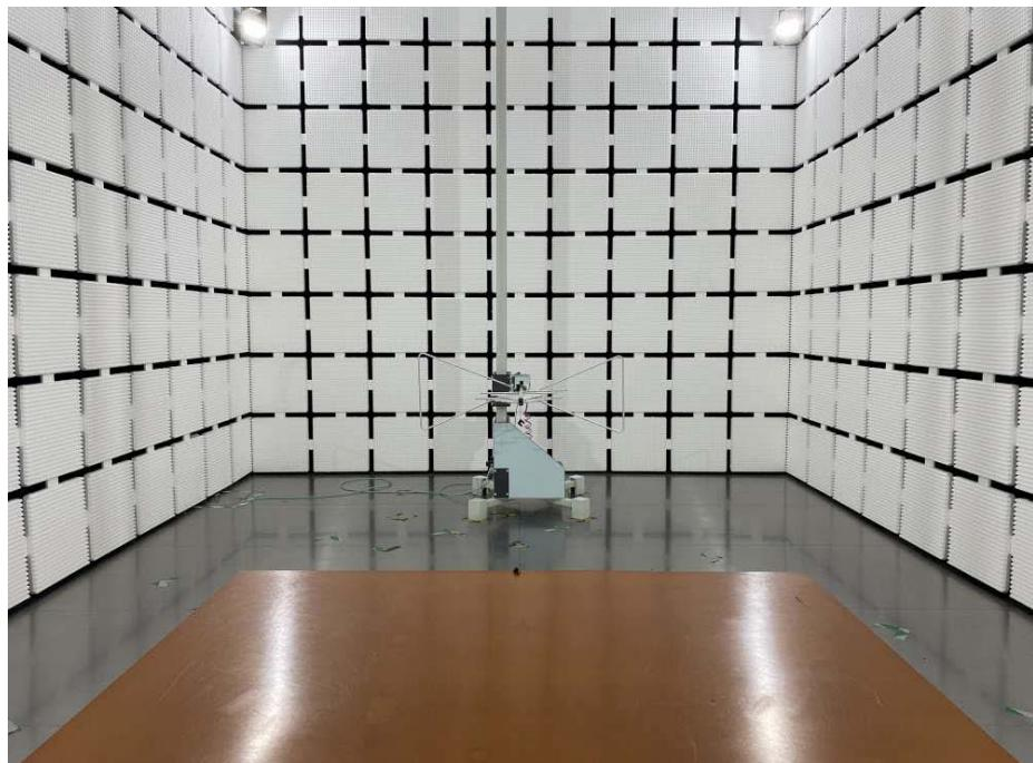
**Radiated Emission Test View Above 1GHz**
