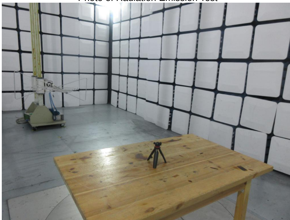
FCC ID:2AXB5-WFC-012 Photo of Radiation Emission Test
