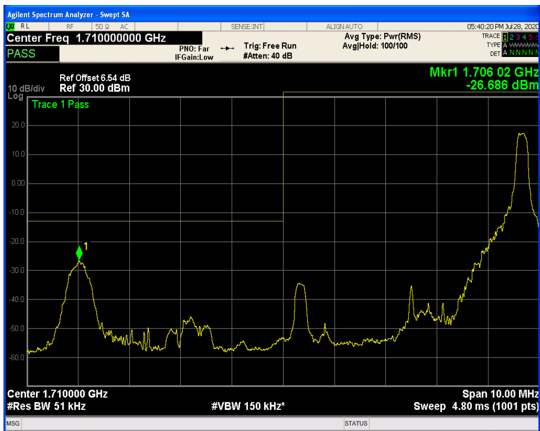
LTE Band4 QAM16 BW=5MHz Channel=19975 RB Size=25 Position=#0
