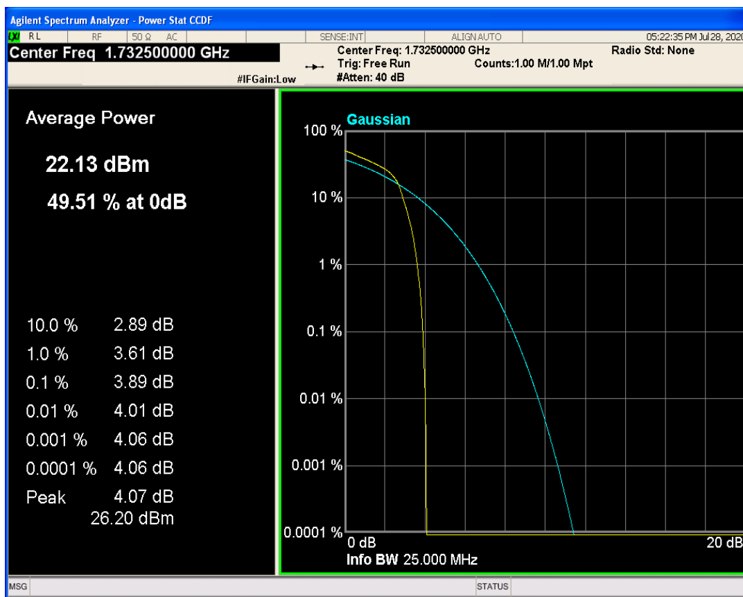
LTE Band4 QPSK BW=3MHz Channel=20175 RB Size=1 Position=#0
