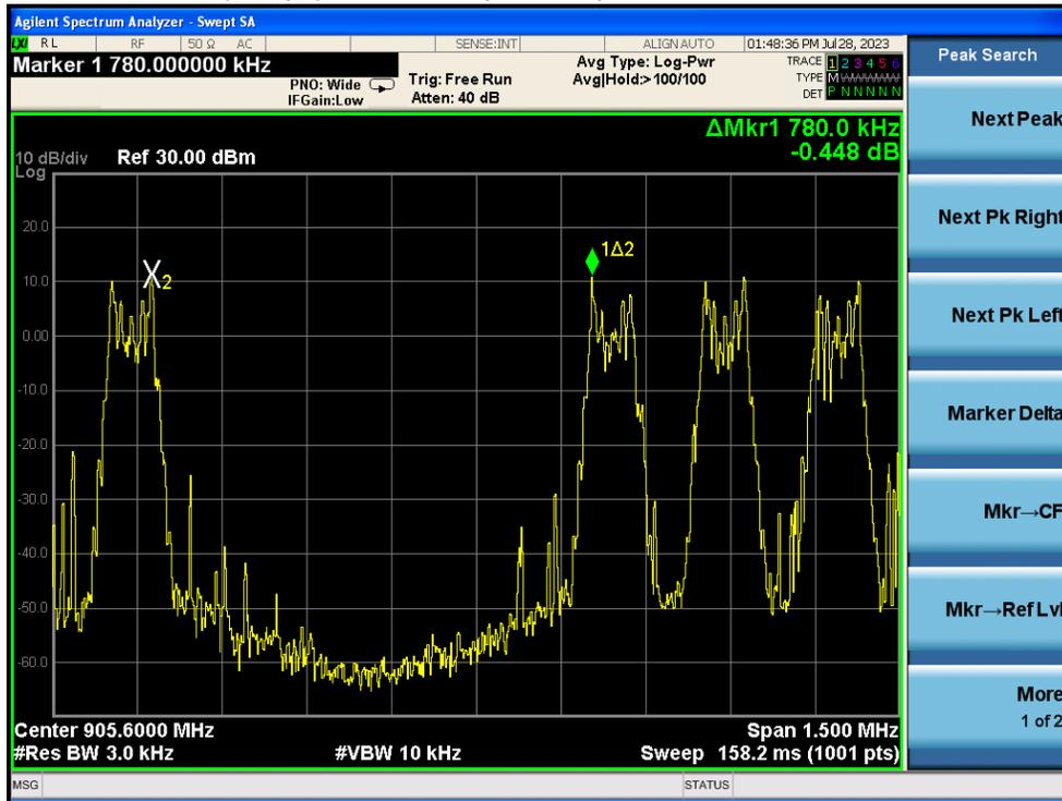
(1Mbps) Channel Separation plot on channel 52-53
