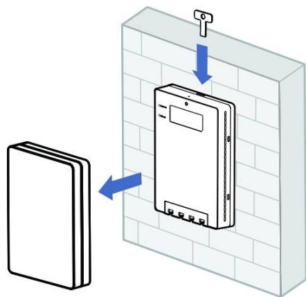
(2) Push the access point upward to remove it from the mounting bracket.
