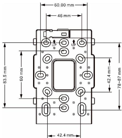
The access point can be installed on various junction boxes, including Chinese-standard and European-standard 86-mm junction boxes, American-standard 118-mm junction box, and South African-standard 120-mm junction box. To mount the access point on a Chinese-standard 86-mm junction box, follow these steps:
