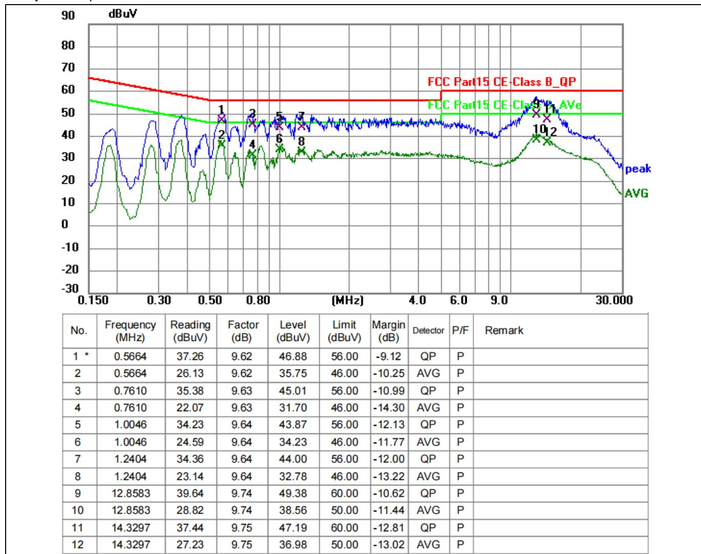
Test phase: N phase IEEE 802.11a TX 5180MHz
