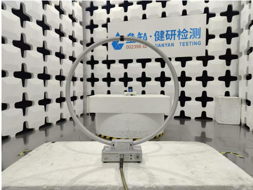
Radiated Spurious Emission 9KHz ~ 30MHz
