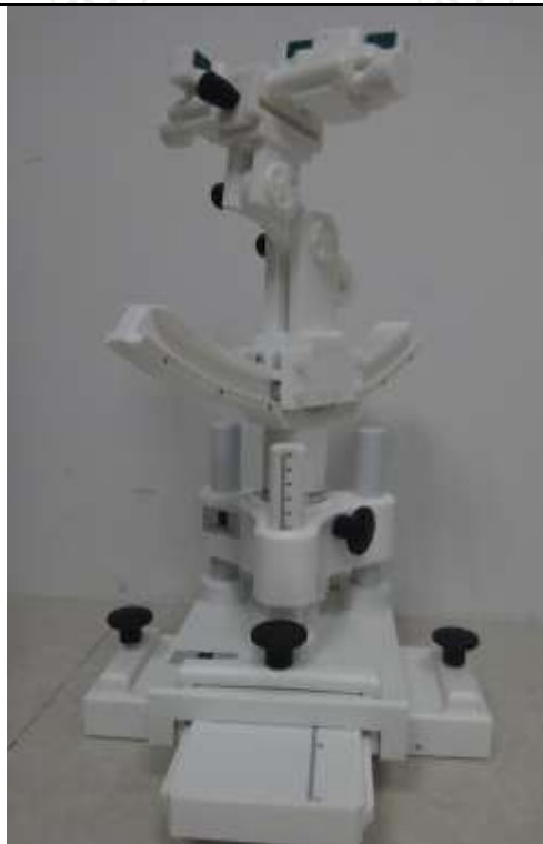
COMOSAR Mobile phone positioning system
