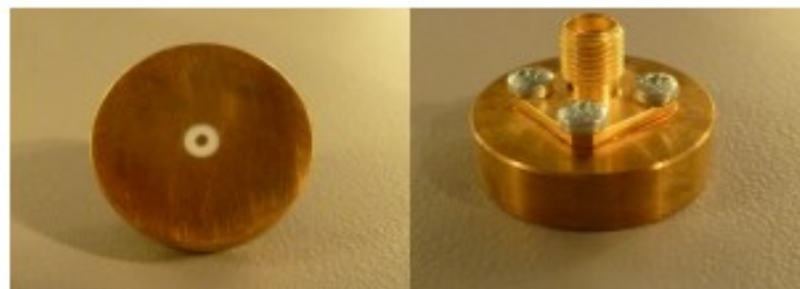
Figure 1 – MVG LIMESAR Dielectric Probe
