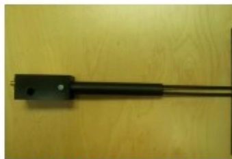
Figure 1 – MVG COMOSAR Validation Dipole
