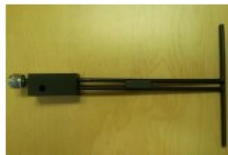
Figure 1 – MVG COMOSAR Validation Dipole
