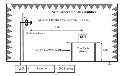
8.2.2 In 3m Anechoic Chamber Test Setup Diagram for frequency above 1GHz
