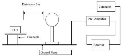
8.2.1 In 3m Anechoic Chamber Test Setup Diagram for below 1GHz
