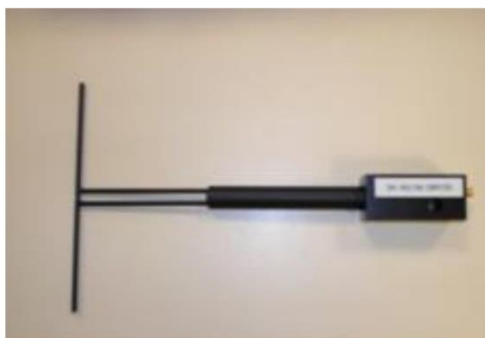
Figure 1 – Satimo COMOSAR Validation Dipole
