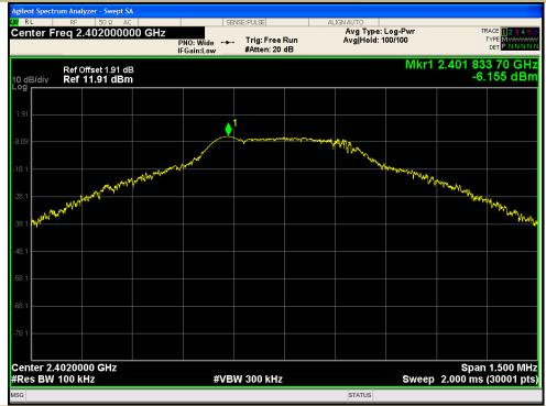
Conduceted Spurious RF Conducted Emission
