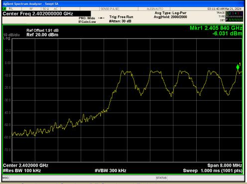
Conduceted Spurious RF Conducted Emission
