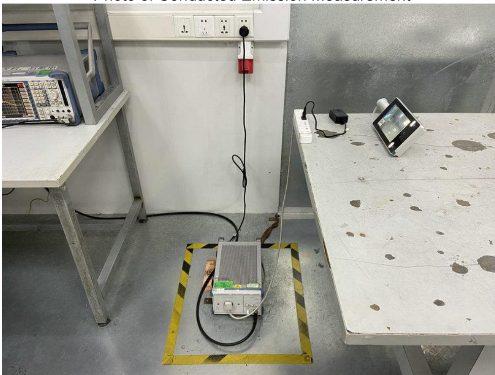
FCC ID: 2AWS-D-V3W Photo of Conducted Emission Measurement
