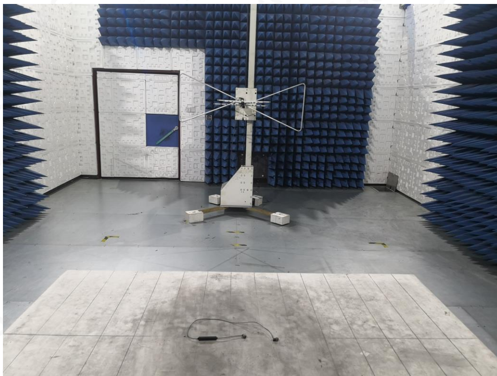
RADIATED EMISSION TEST SETUP ABOVE 1GHZ
