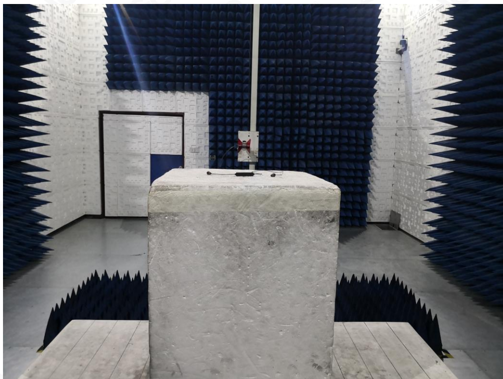
RADIATED EMISSION TEST SETUP ABOVE 1GHZ
