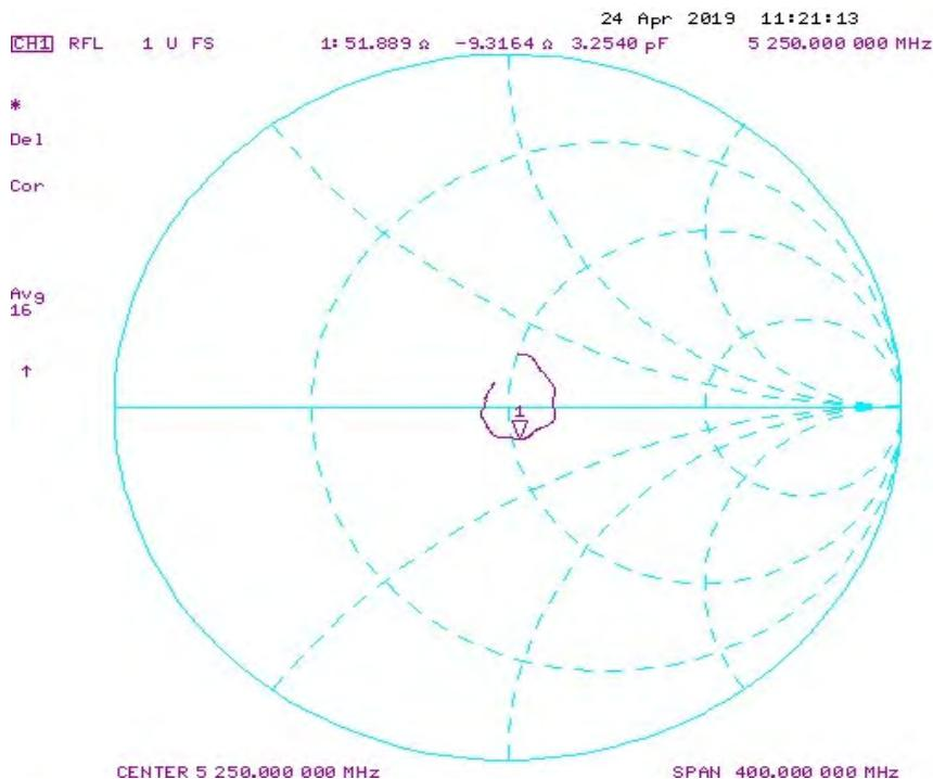
**5GHz Dipole Extended Calibration**
