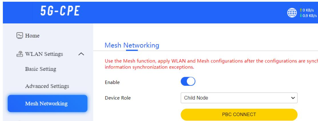
After waiting for about 40 seconds, the WiFi icon in the sub node status bar will display the gray 'Mesh' label. The signal light on the child node device will remain solid yellow, indicating that the configuration of the sub node is complete.
