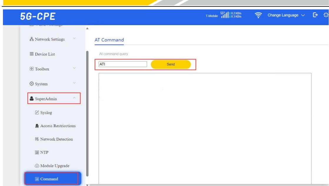
After receiving the command, the device executes the relevant instructions, generates the corresponding information, and sends it back to the configuration page.
