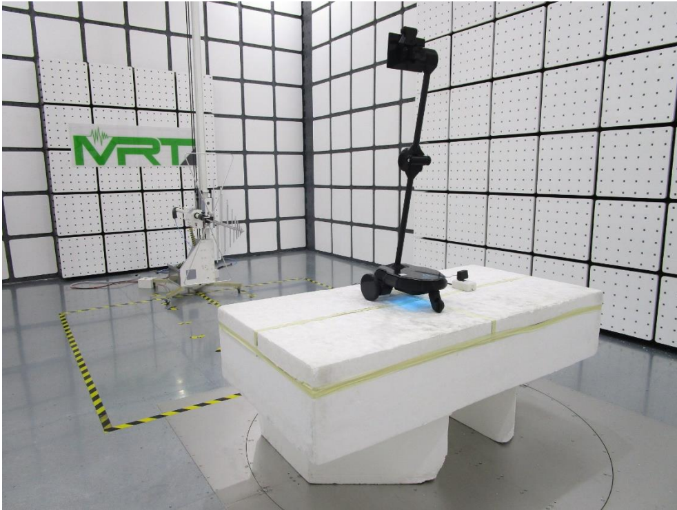
Description: Radiated Emission Test Setup for 30MHz~1GHz
