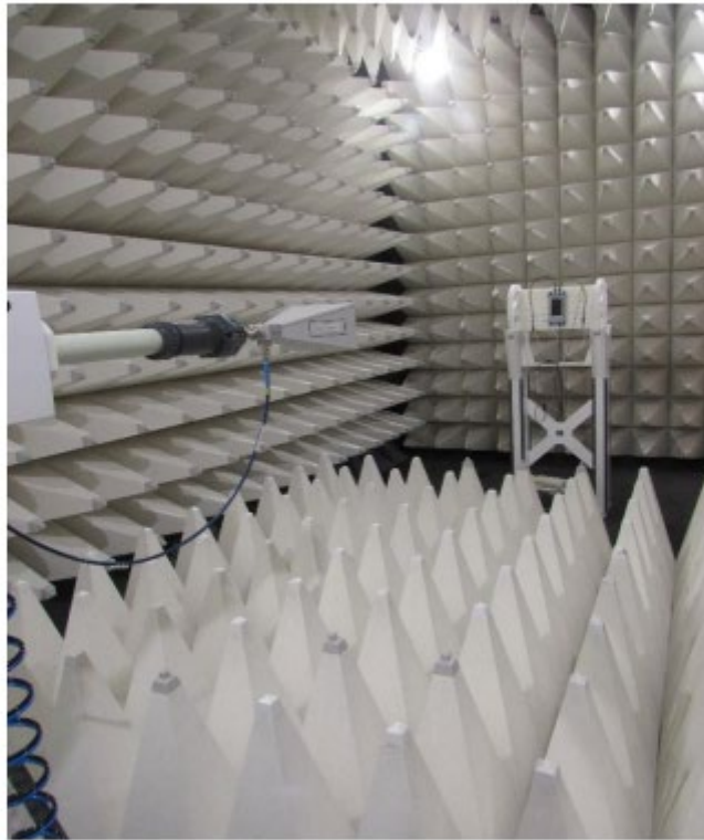
Setup for measurements above 1 GHz
