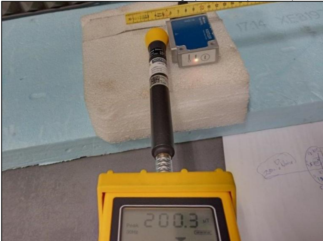
Photo 4: Test Position - WC- H- field strength (ELT400 3cm 2 probe, touch)
