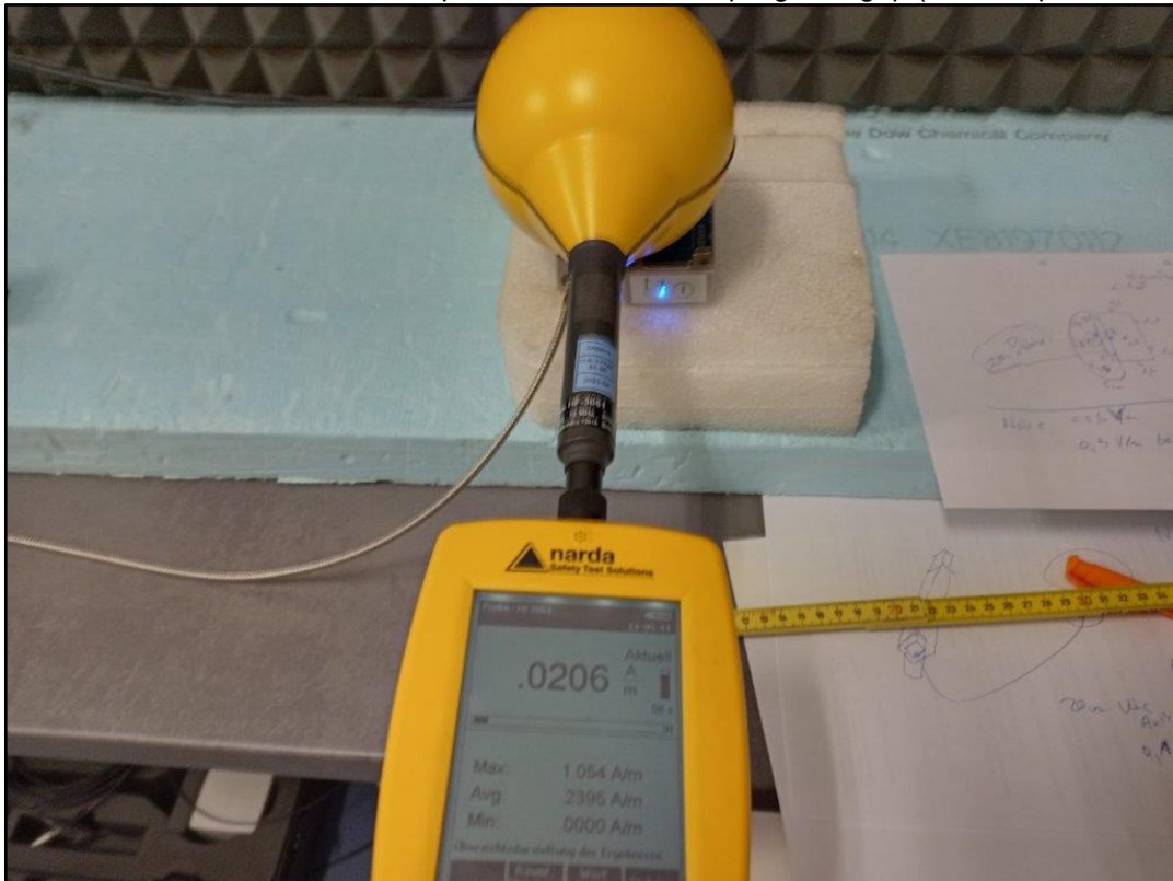
Photo 8: Test Position - H- field at top side of the WPT coupling field gap (HF6091 probe, touch)
