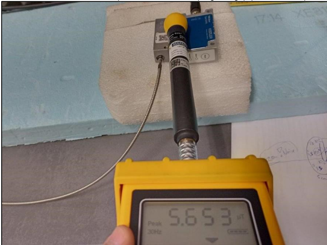
Photo 5: Test Position - WC- H- field top side of the WPT coupling field gap (ELT400 3cm 2 probe, touch)
