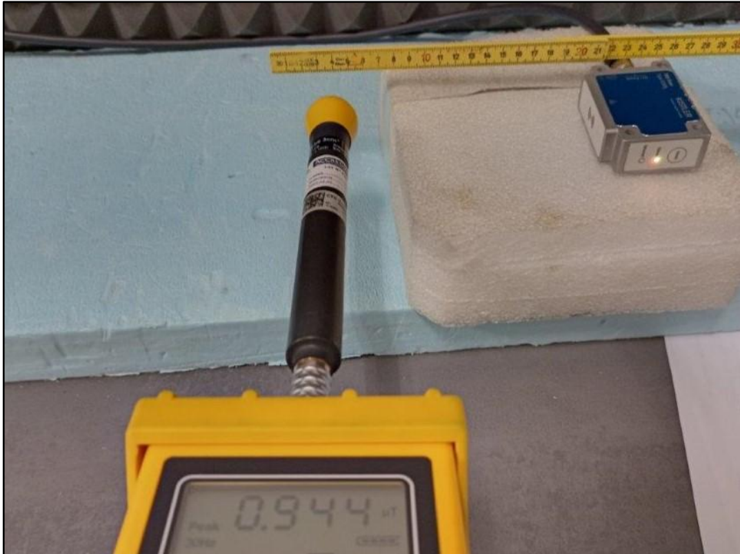
Photo 3: Test Position - Noise < 1 \mu T already at 10 to 20 cm distance (ELT400 3cm 2 probe)
