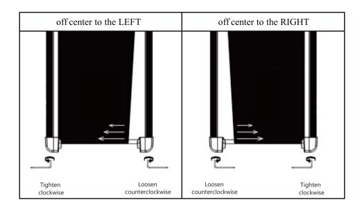
To determine left-right orientation, stand at the rear of the treadmill, facing the display. Use the provided hex wrench to make all belt adjustments on the rear bolt.
