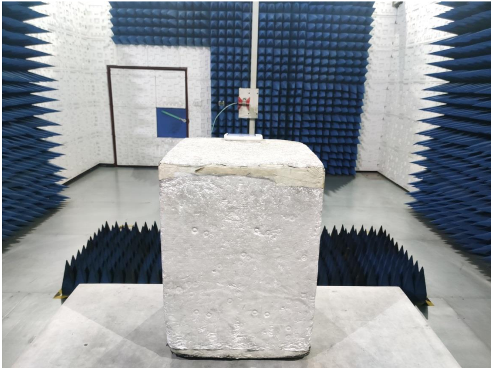
RADIATED EMISSION TEST SETUP ABOVE 1GHz
