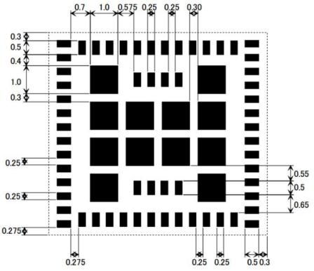
To avoid the short-circuit between the side shielding and a solder on the module land after the reflow, please locate the module land at 0.2mm away from module outline as above figure.
