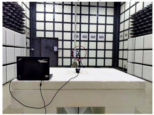
Radiated Emission Set up Photos (30MHz~1GHz)
