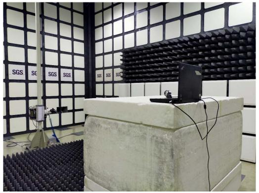
Radiated Emission Set up Photos (Front View)
