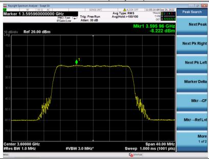
EIRP PSD=-8.22-2.3+3=-7.52dBm/MHz, loss of Cable and Splitter is 3dB, Antenna gain is -2.3dBi.
