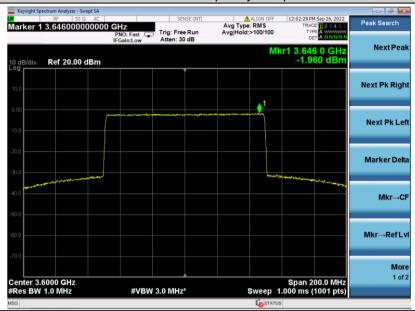
EIRP PSD=-1.96-2.3+3=-1.26dBm/MHz, loss of Cable and Splitter is 3dB, Antenna gain is -2.3dBi.
