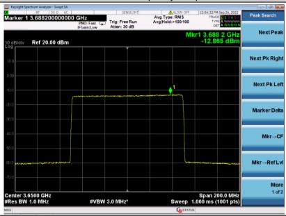
EIRP PSD=-12.865-2.3+3=-12.165dBm/MHz, loss of Cable and Splitter is 3dB, Antenna gain is -2.3dBi.
