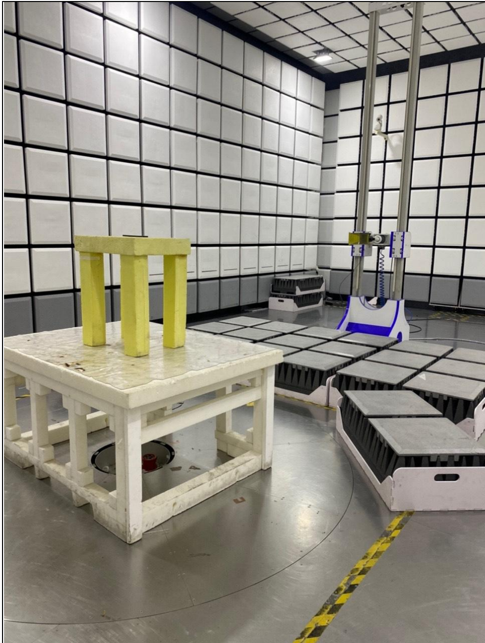
RADIATED EMISSION TEST (Above1GHz)
