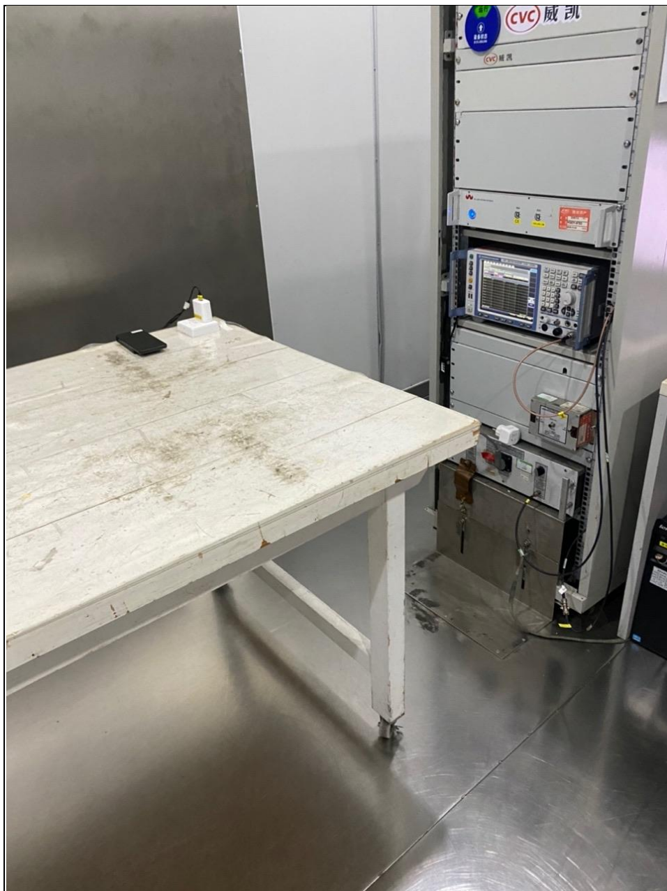
CONDUCTED EMISSION TEST
