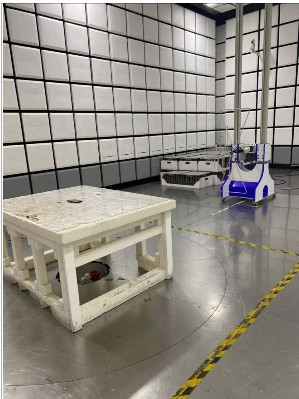
RADIATED EMISSION TEST (Below 1GHz)
