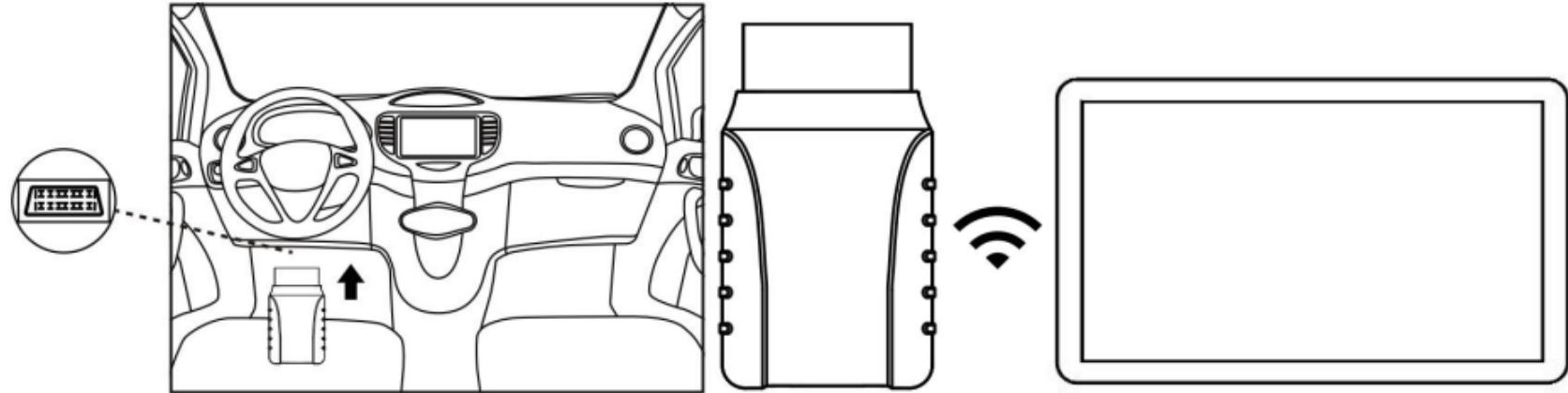
Plug the Wireless Diagnostics Module to vehicle's DLC port first, then connect the device via Wi-Fi.
