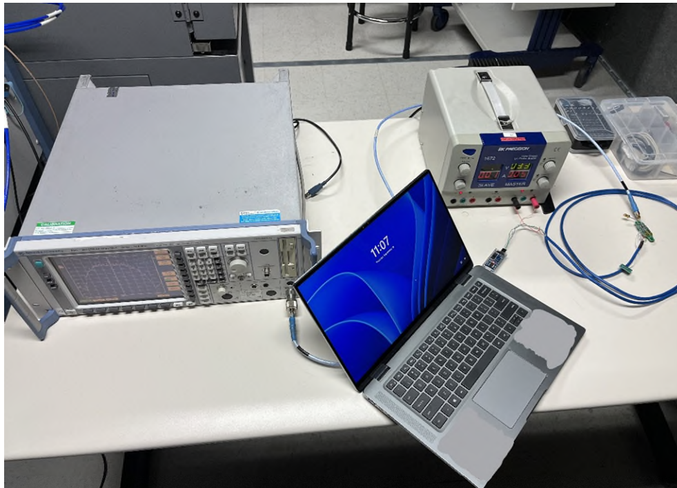
Photo 7: Test setup for conducted test, e.g. bandwidth
