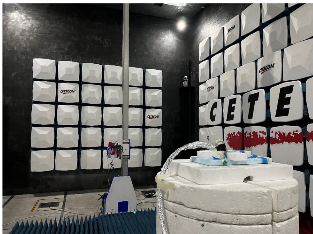
Photo 4: Emissions in frequency range 3-18 GHz
