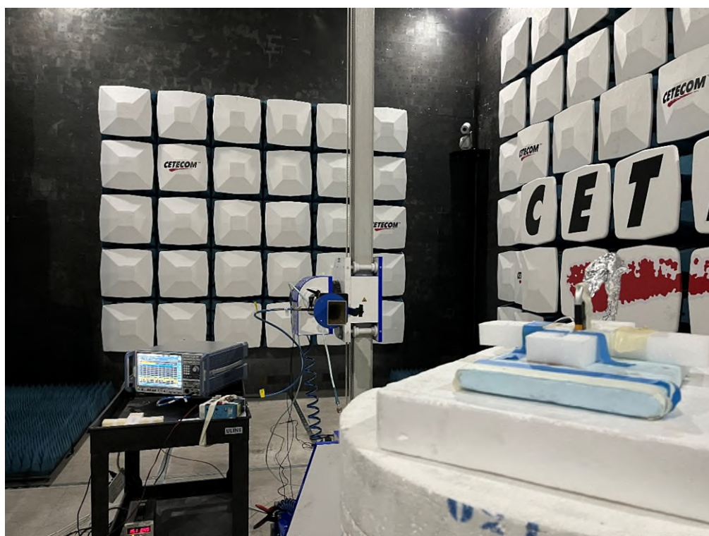
Photo 6: Emissions in frequency range 26-40 GHz
