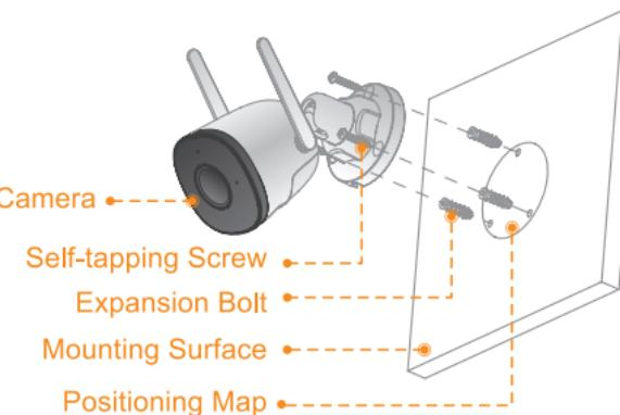
**Step1** Drill screw holes on the mounting surface as the positioning map shows, and then put in the expansion bolts.
